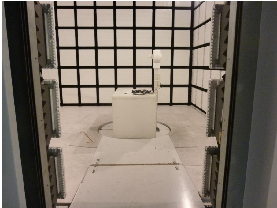
Photo 8: EUT at the anechoic chamber, loop antenna test setup
