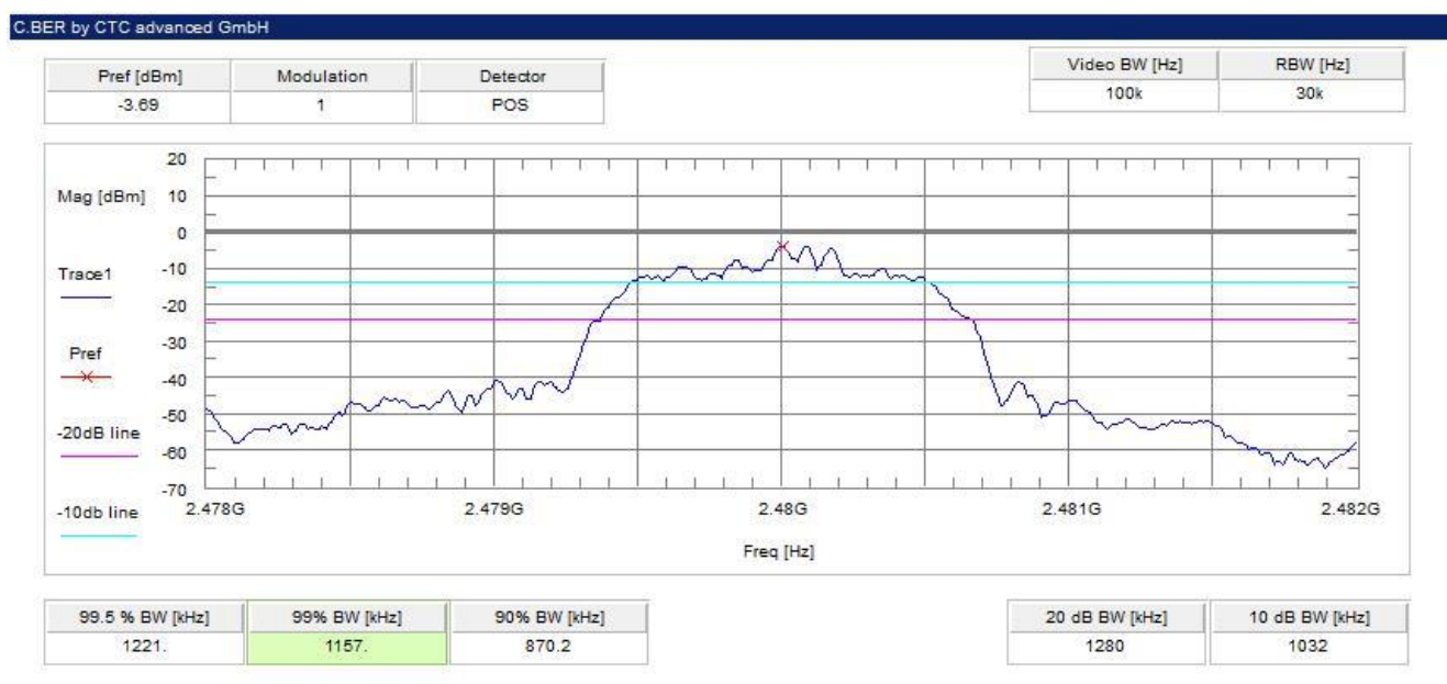
Plot 6: highest channel – 2480 MHz, Pi / DQPSK modulation
