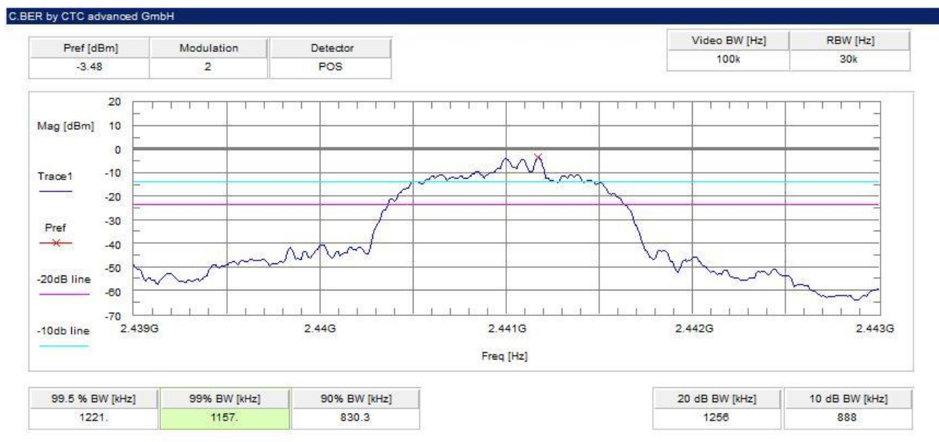
Plot 8: middle channel – 2441 MHz, 8 DPSK modulation
