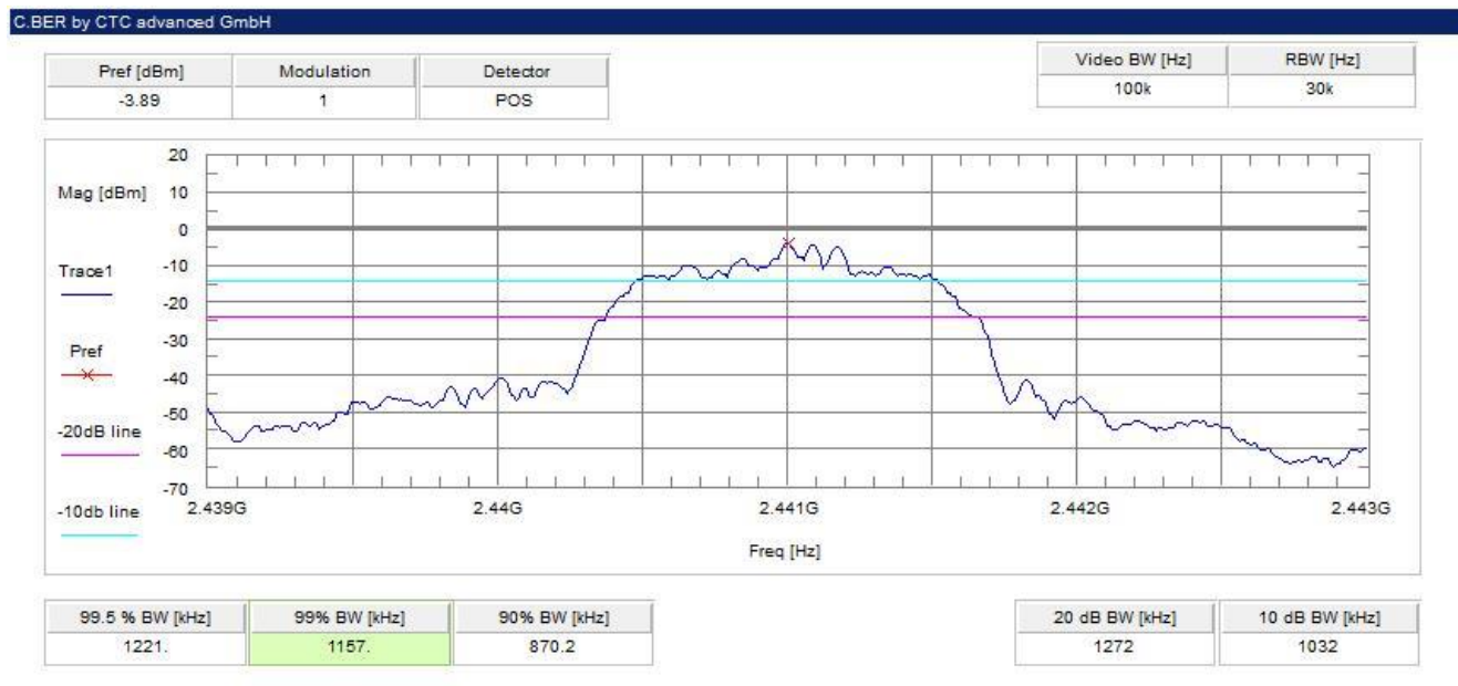
Plot 5: middle channel – 2441 MHz, Pi / DQPSK modulation
