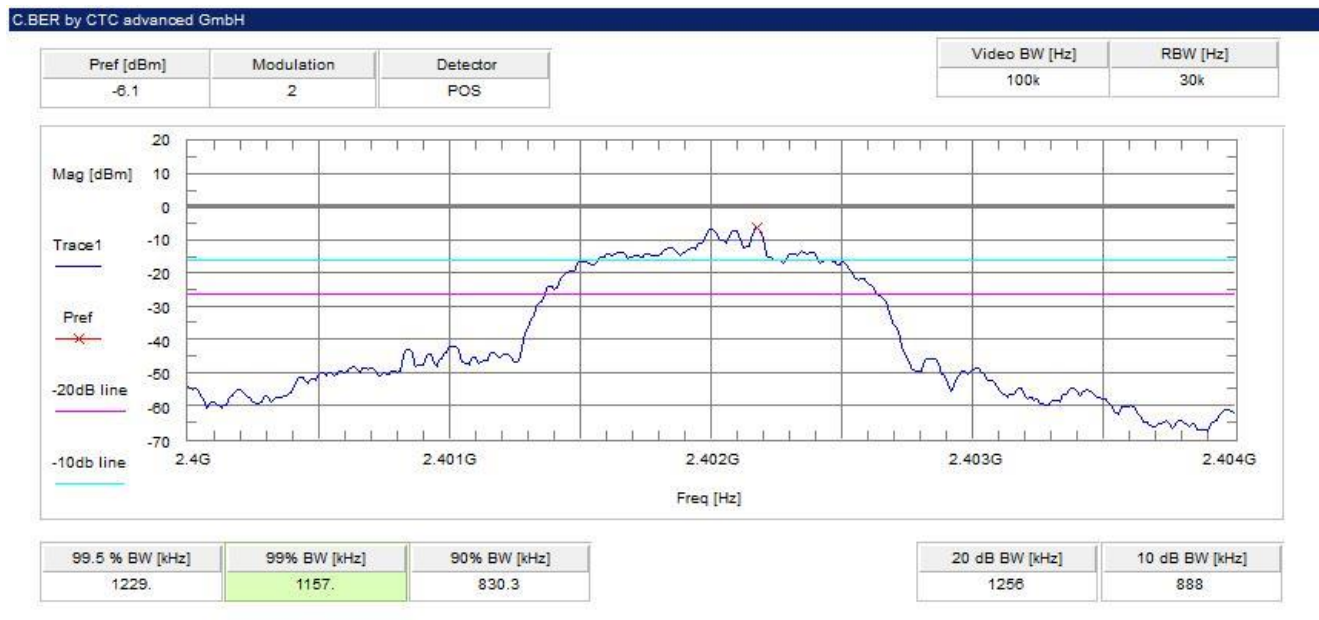
Plot 7: lowest channel – 2402 MHz, 8 DPSK modulation
