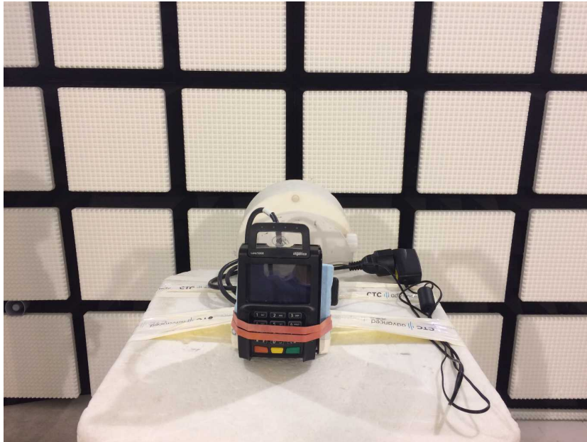
Photo 1: RSE test setup >1GHz
