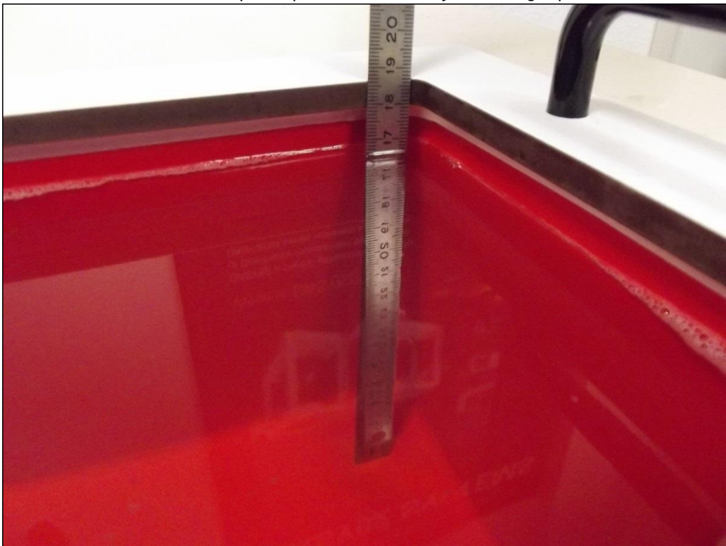
Photo 2: Liquid depth 1900 MHz body simulating liquid
