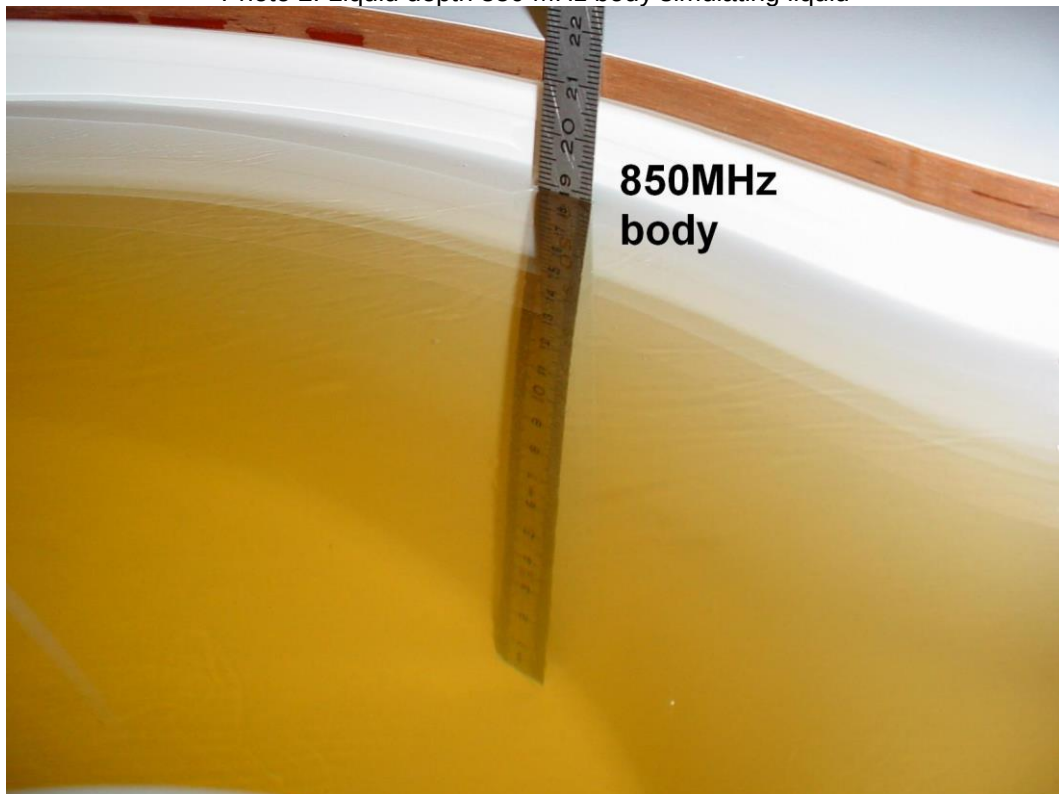
Photo 2: Liquid depth 850 MHz body simulating liquid
