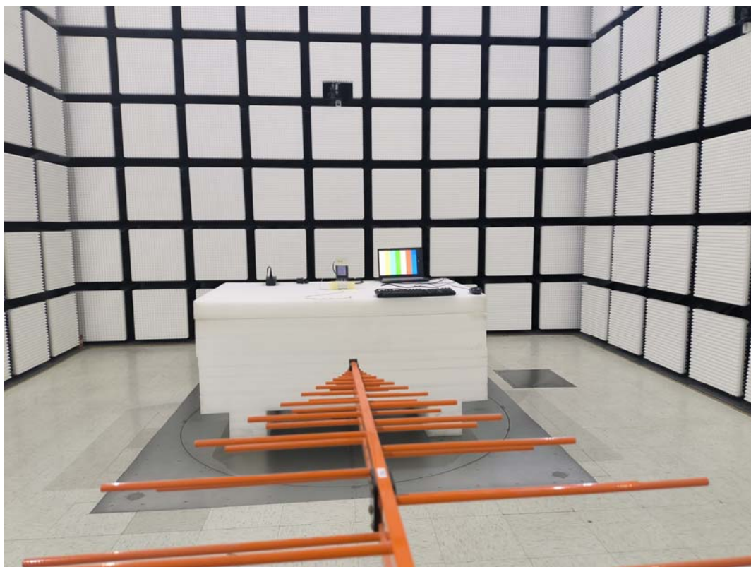
Radiated Emission Below 30MHz View -Parallel
