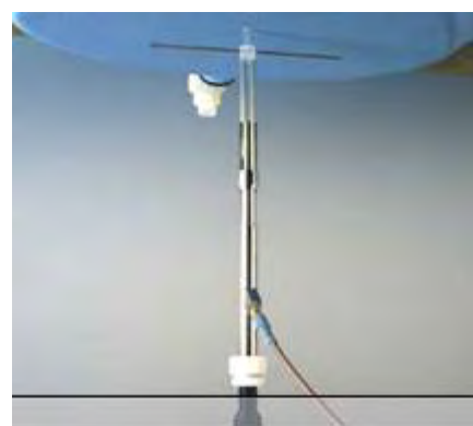
Photograph of the dipole Antenna
