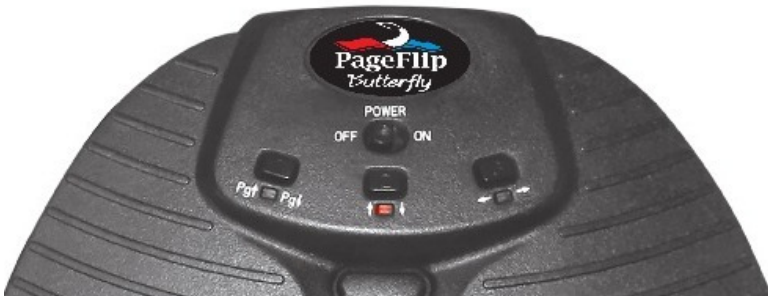
Figure 2: Top view of PageFlip Butterfly control panel.
