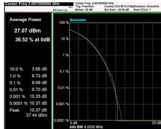
Channel: MIDDLE, Modulation: 64QAM, BW=5MHz, CCDF
