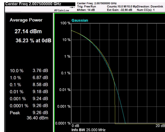
Channel: MIDDLE, Modulation: 256QAM, BW=10MHz, CCDF
