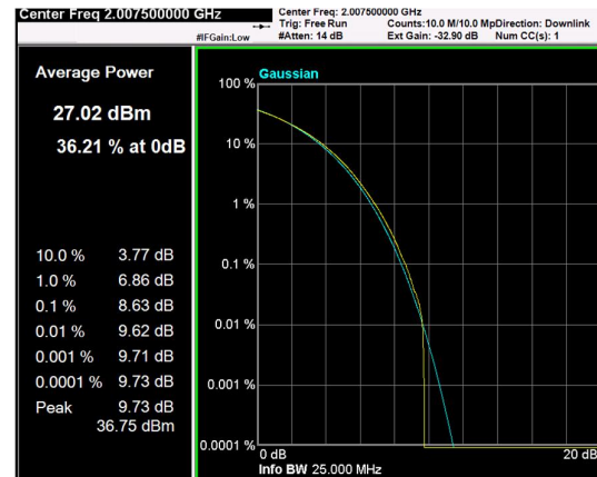
Channel: MIDDLE, Modulation: 64QAM, BW=15MHz, CCDF
