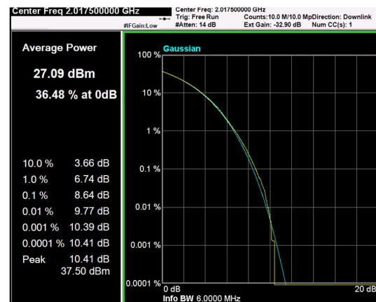
Channel: TOP, Modulation: 64QAM, BW=5MHz, CCDF
