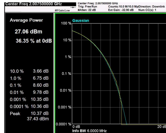
Channel: MIDDLE, Modulation: 16QAM, BW=5MHz, CCDF
