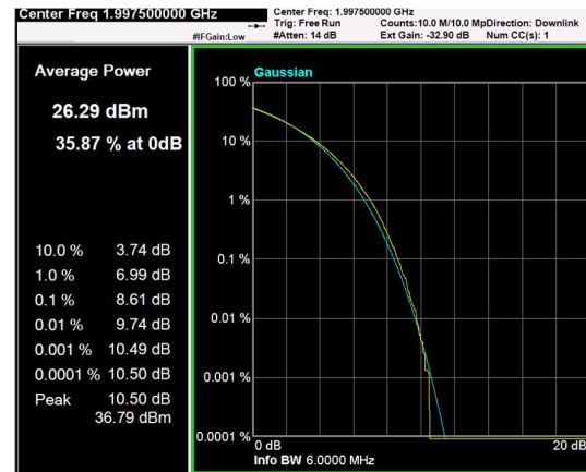
Channel: BOTTOM, Modulation: 64QAM, BW=5MHz, CCDF
