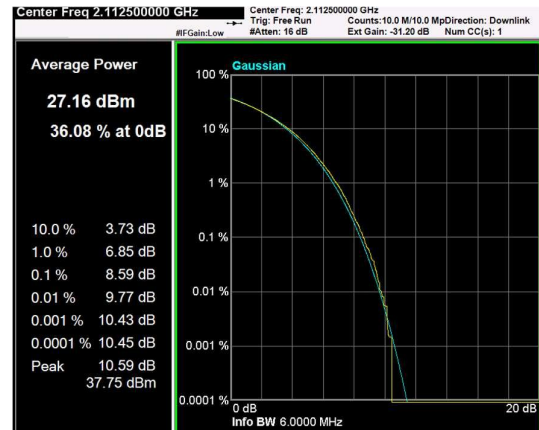
Channel: BOTTOM, Modulation: QPSK, BW=5MHz, CCDF
