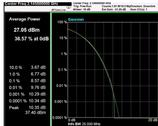
Channel: MIDDLE, Modulation: 256QAM, BW=5MHz, CCDF
