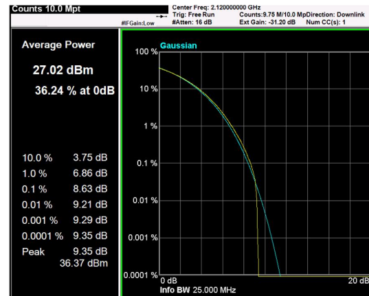
Channel: BOTTOM, Modulation: 256QAM, BW=20MHz, CCDF
