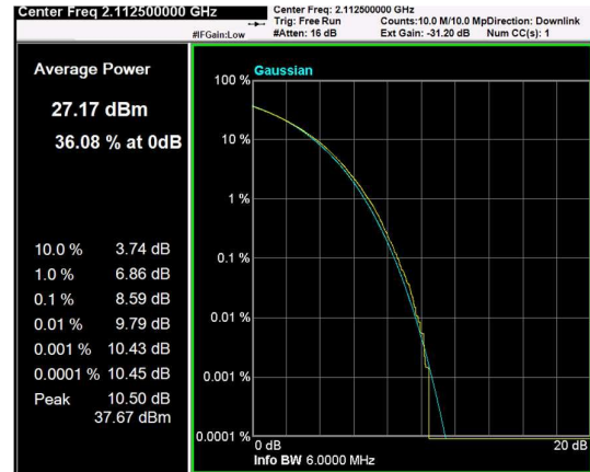
Channel: BOTTOM, Modulation: 16QAM, BW=5MHz, CCDF
