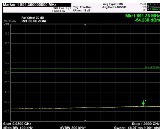
Channel: TOP, Modulation: 256QAM, BW=20MHz, Range: Lower
