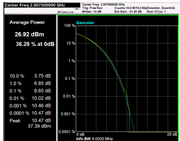
Channel: MIDDLE, Modulation: 256QAM, BW=5MHz, CCDF
