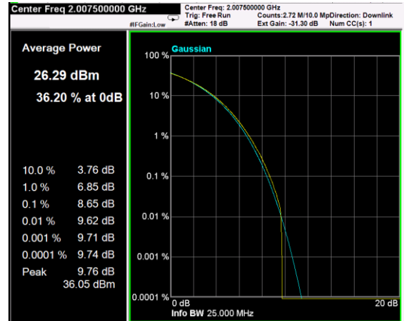
Channel: BOTTOM, Modulation: QPSK, BW=15MHz, CCDF
