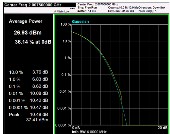
Channel: MIDDLE, Modulation: 16QAM, BW=5MHz, CCDF
