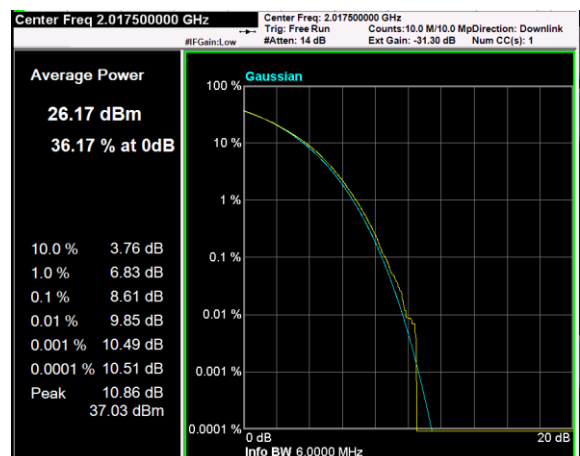
Channel: TOP, Modulation: QPSK, BW=5MHz, CCDF
