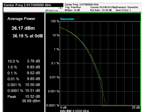
Channel: TOP, Modulation: 256QAM, BW=5MHz, CCDF
