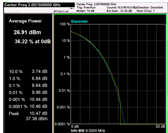
Channel: MIDDLE, Modulation: QPSK, BW=5MHz, CCDF
