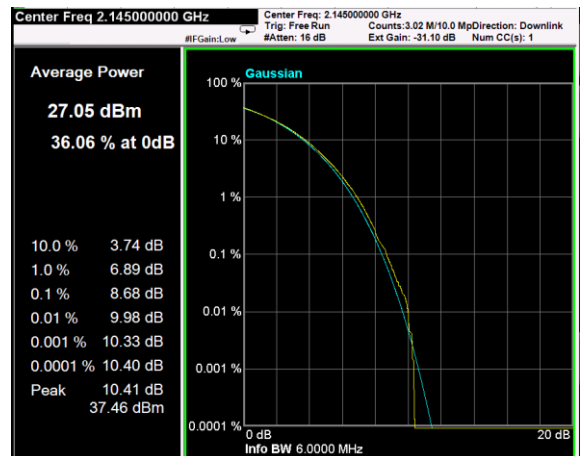
Channel: MIDDLE, Modulation: 64QAM, BW=5MHz, CCDF
