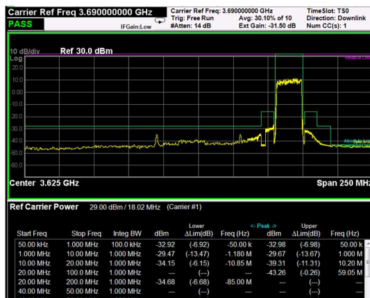
High Band Edge, 1 Carrier, Modulation: 64QAM, BW=20MHz
