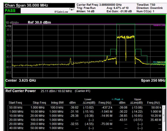
High Band Edge, 2 Carrier, Modulation: 16QAM, BW=15MHz
