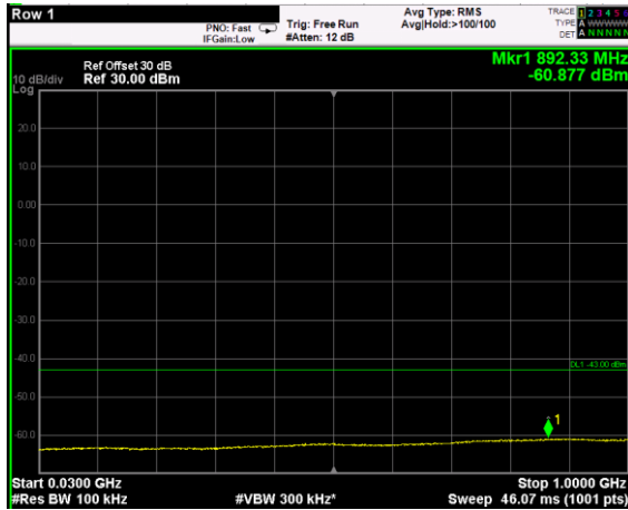
Channel: TOP, Modulation: 256QAM, BW=10MHz, Range: 30MHz - 1GHz
