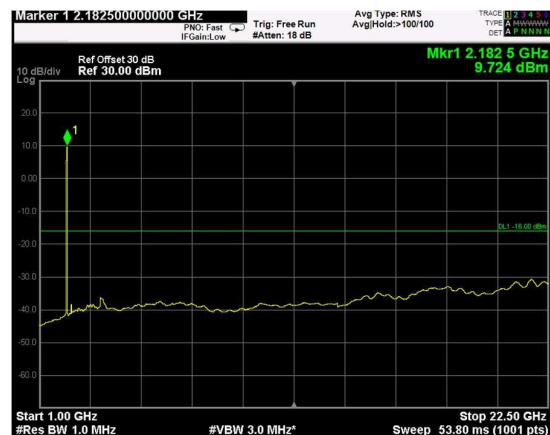
Channel: TOP, Modulation: 64QAM, BW=15MHz, Range: Upper
