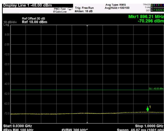
Channel: TOP, Modulation: 64QAM, BW=5MHz, Range: Lower
