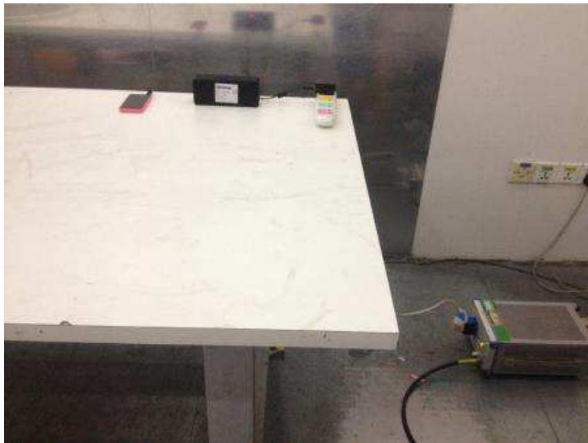
Photograph 4: Set-up for Conducted Emissions
