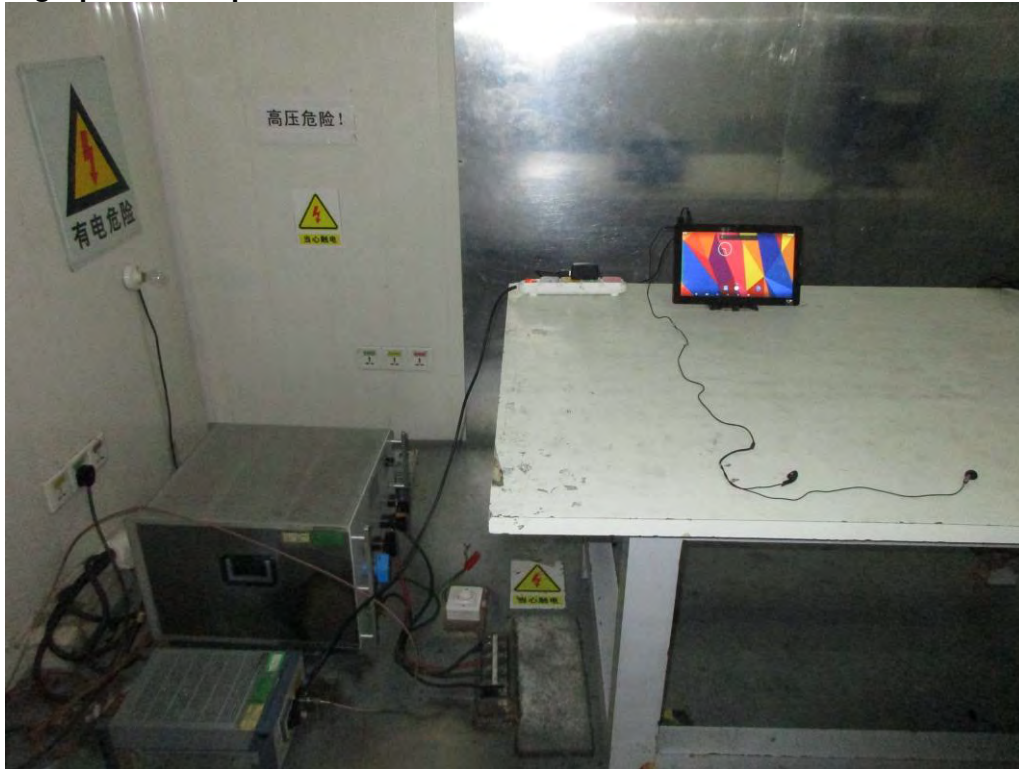
Photograph 5: Set-up for Conducted Emission
