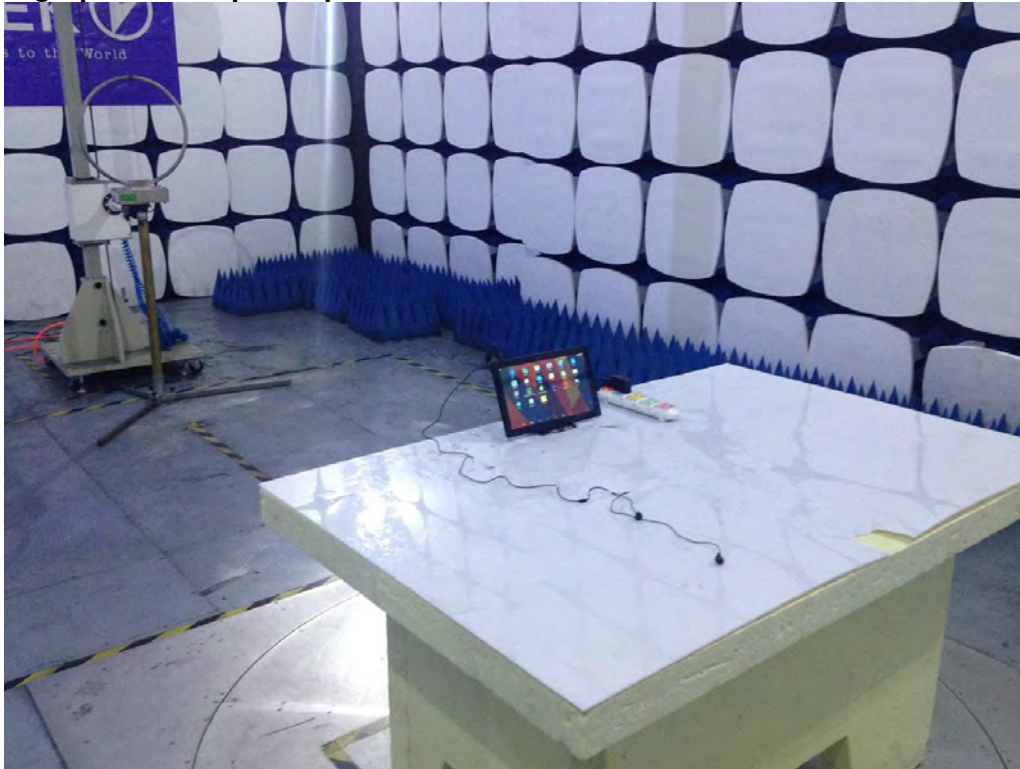
Photograph 2: Set-up for Spurious Emissions for 30 - 1000MHz
