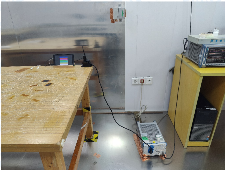
Photo of Setup for Radiated Emission (30MHz~1GHz)
