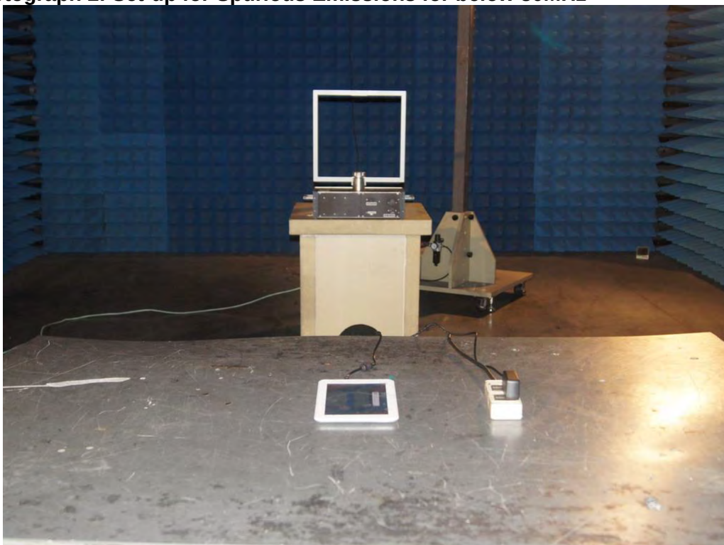
Photograph 2: Set-up for Spurious Emissions for below 30MHz
