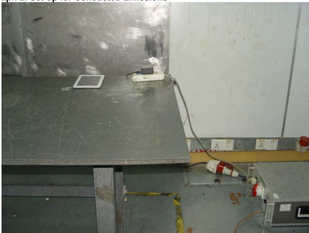
Photograph 2: Set-up for Spurious Emissions for below 30MHz
