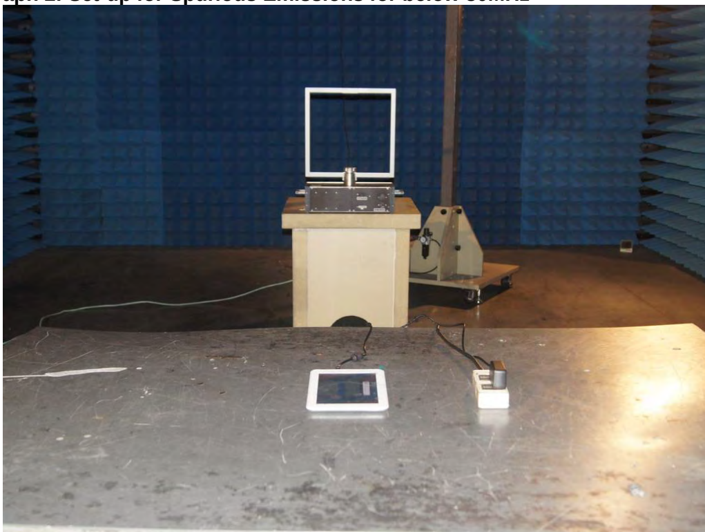
Photograph 2: Set-up for Spurious Emissions for below 30MHz
