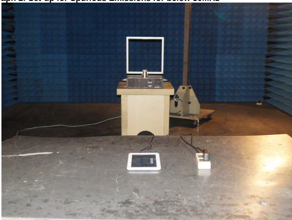
Photograph 2: Set-up for Spurious Emissions for below 30MHz
