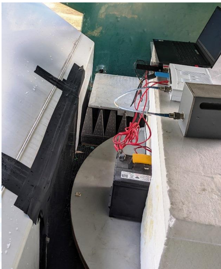
Biconical Antenna pointing towards Test Enclosure.
