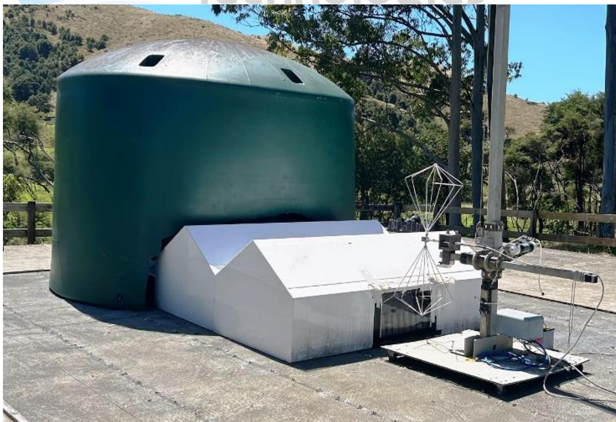
Biconical Antenna pointing towards Test Enclosure.
