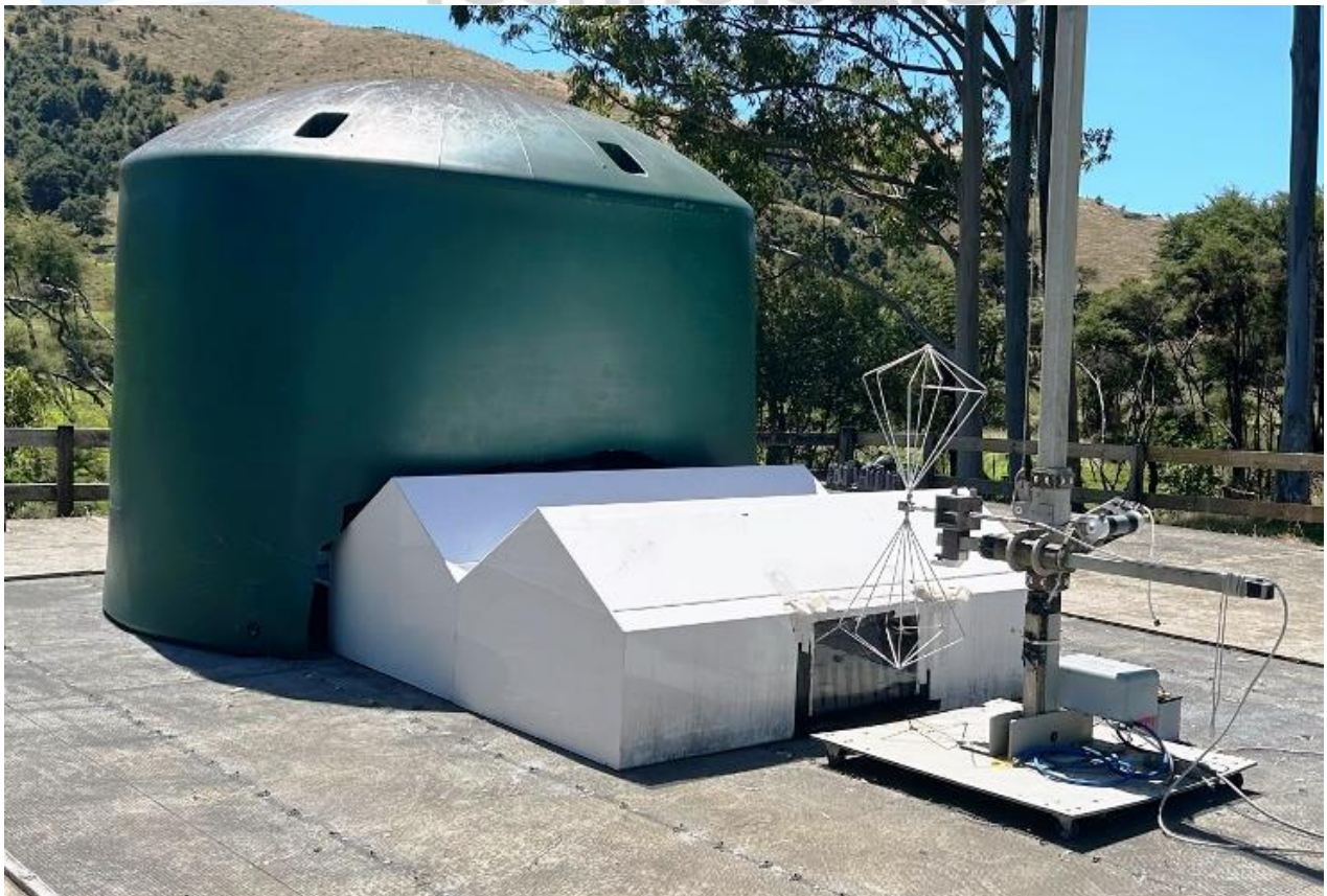
Biconical Antenna pointing towards Test Enclosure.
