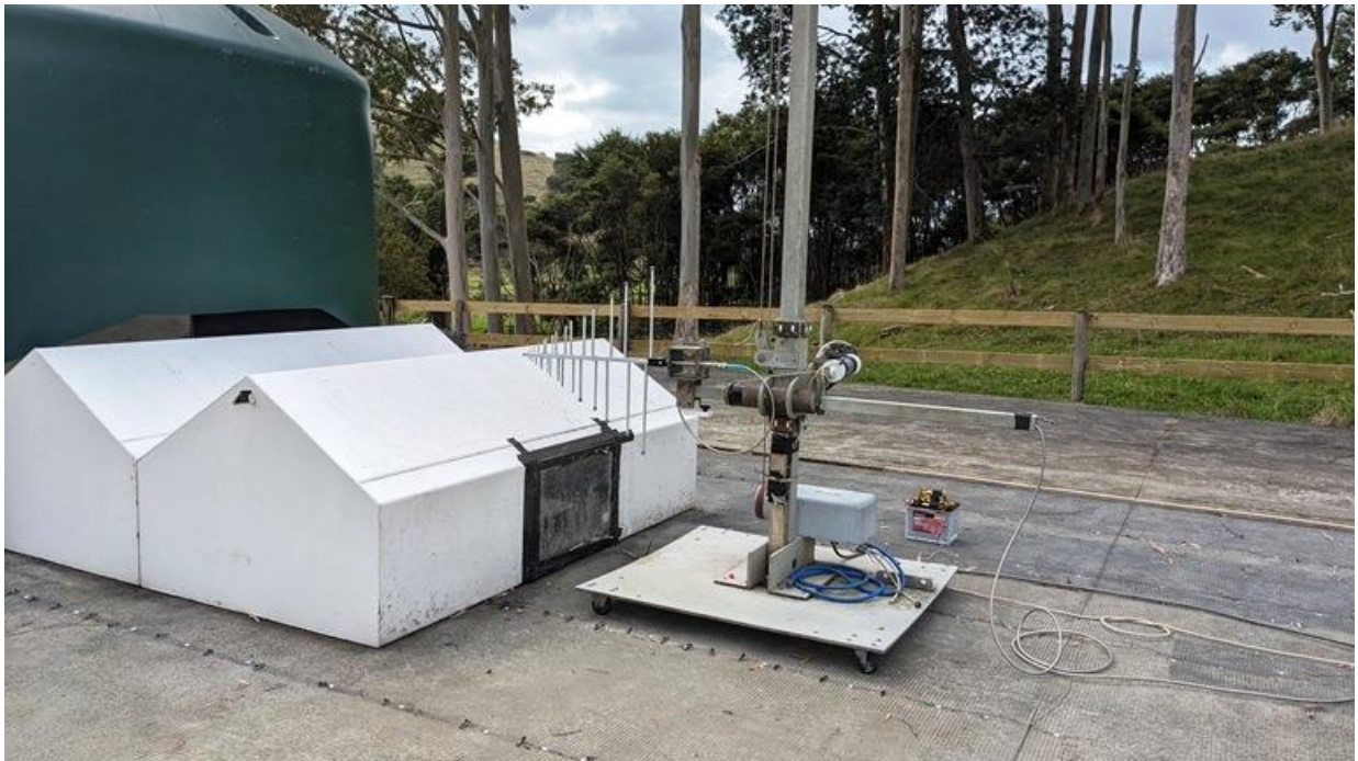
Horn Antenna pointing towards Test Enclosure.
