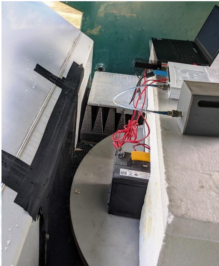
Biconical Antenna pointing towards Test Enclosure.
