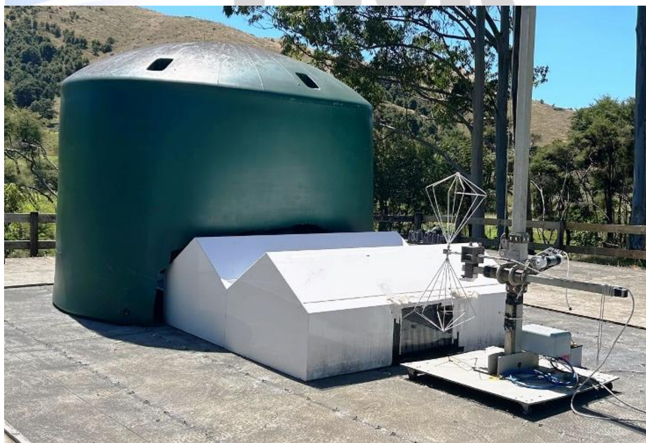
Biconical Antenna pointing towards Test Enclosure
