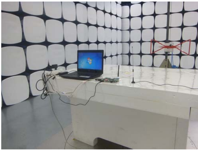
Radiated Spurious Emissions Test Setup Below 1GHz
