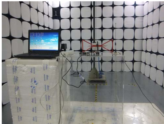
Radiated Spurious Emissions Test Setup Below 1GHz - 2
