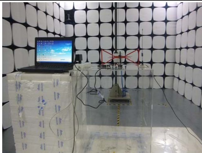
Radiated Spurious Emissions Test Setup Below 1GHz - 2
