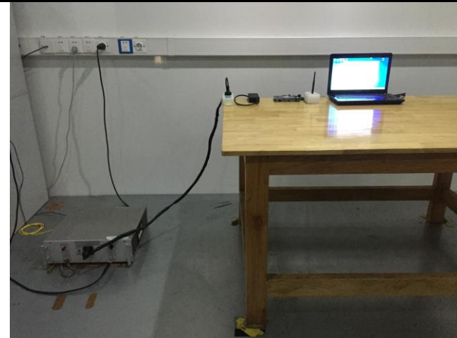
Conducted Emissions Test Setup Front View
