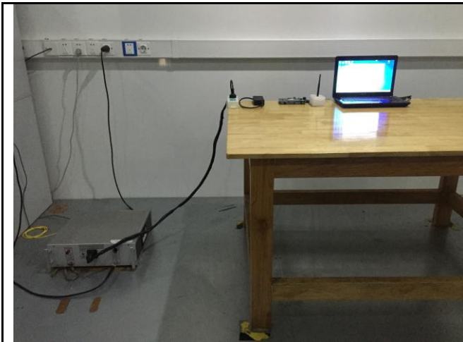
Conducted Emissions Test Setup Front View
