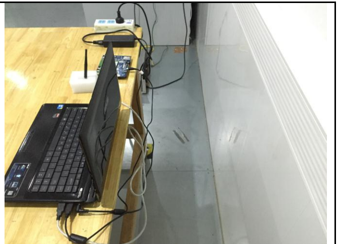
Conducted Emissions Test Setup Side View
