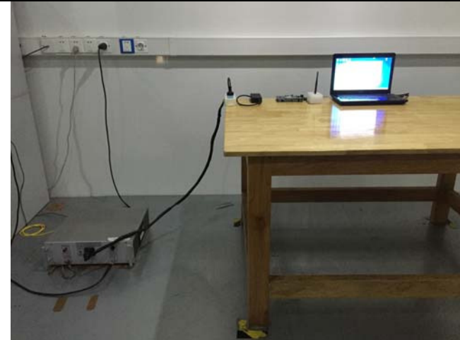
Conducted Emissions Test Setup Front View
