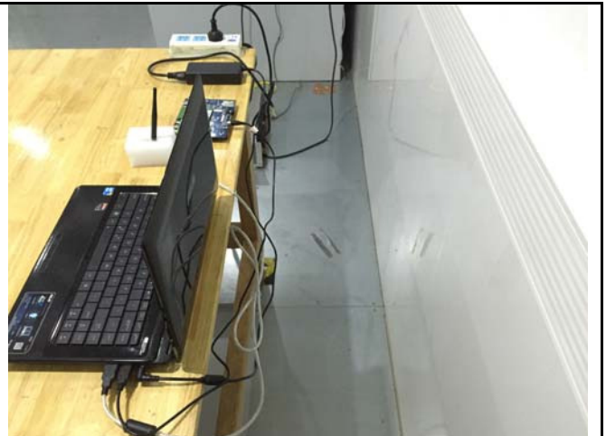
Conducted Emissions Test Setup Side View
