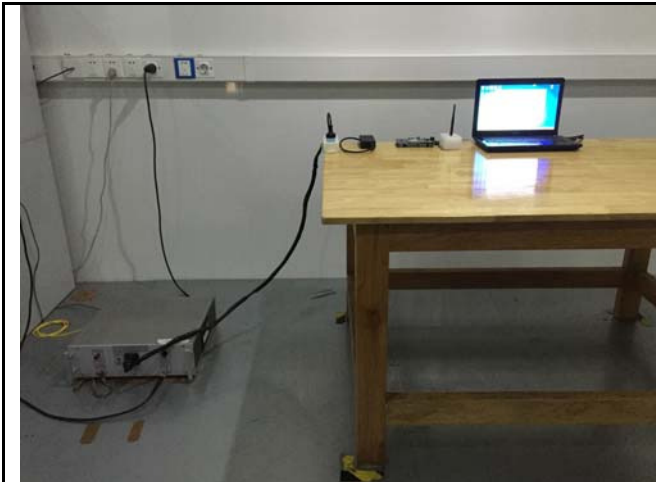
Conducted Emissions Test Setup Front View
