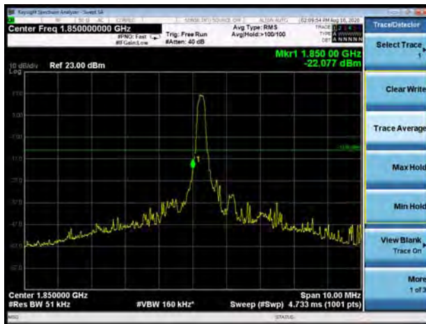
LTE Band 2 1.4MHz QPSK 100%RB CH-Low
