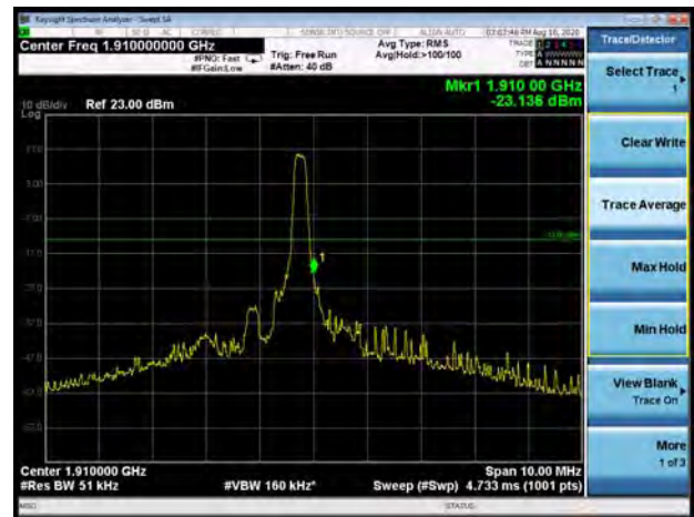
LTE Band 2 1.4MHz QPSK 100%RB CH-High
