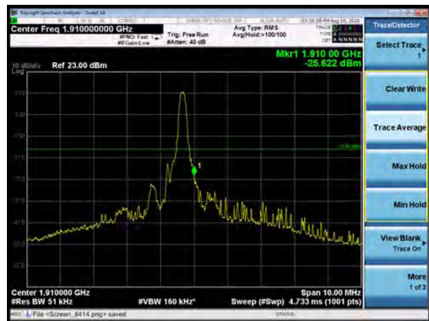
LTE Band 2 5MHz 16QAM 100%RB CH-High
