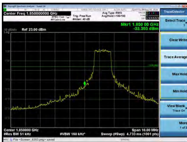
LTE Band 2 15MHz QPSK 1RB CH-Low
