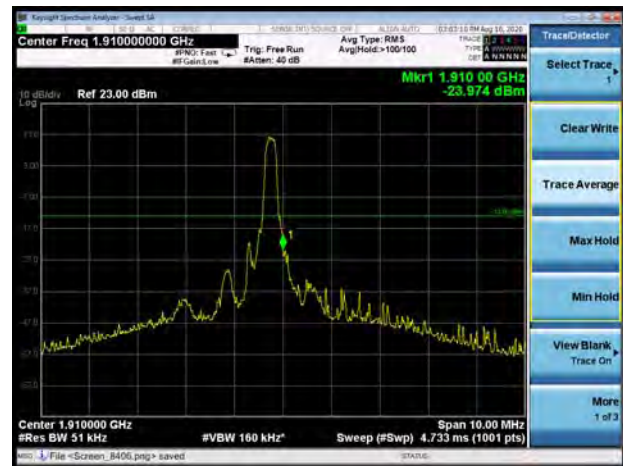
LTE Band 2 1.4MHz 16QAM 100%RB CH-High
