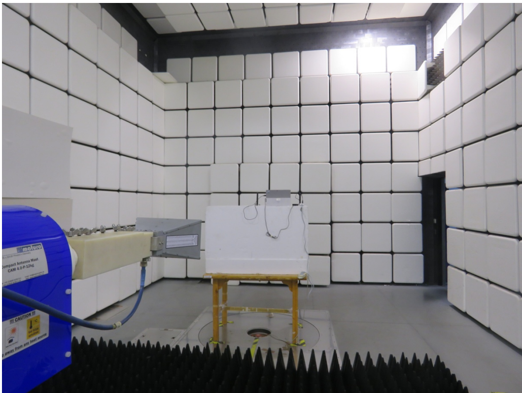
Radiated Spurious Emissions Test setup
