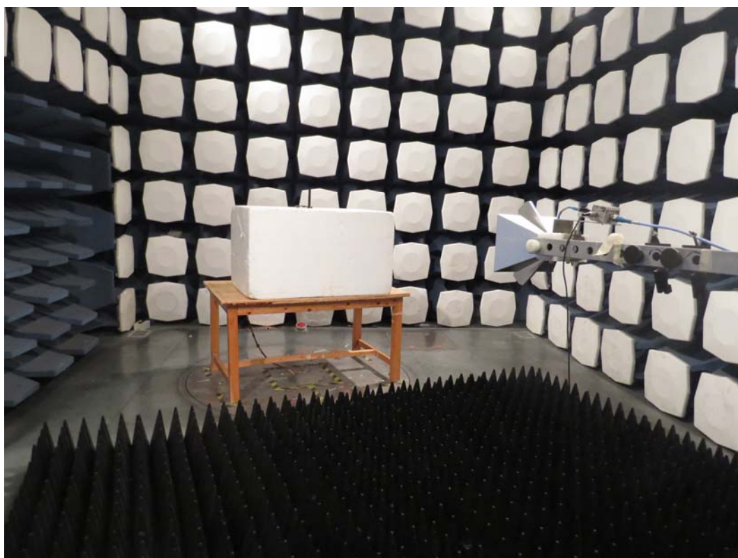
Picture 2 Radiated Spurious Emissions Test setup
