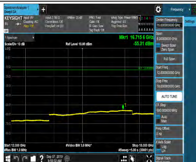
LTE Band 2_3MHz_QPSK_19185_1RB#0_Range1:0.009~0.15MHz_-63.99_PASS
