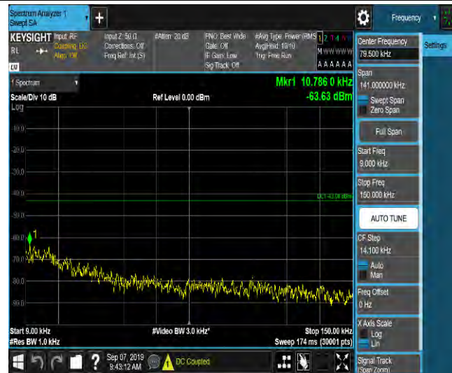
LTE Band 2_15MHz_16QAM_18900_1RB#0_Range2:0.15~30MHz_-59.76_PASS
