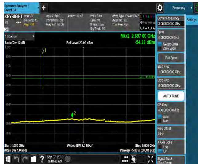
LTE Band 2_3MHz_16QAM_18900_1RB#0_Range5:5000~12000MHz_-65.69_PASS
