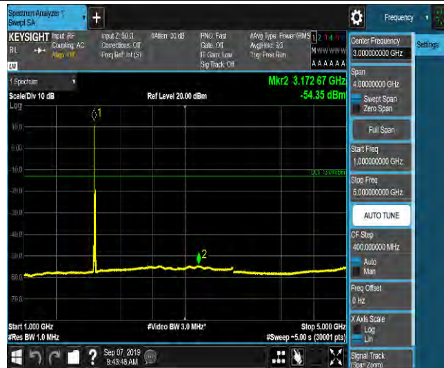
LTE Band 2_15MHz_16QAM_18900_1RB#0_Range5:5000~12000MHz_-65.75_PASS
