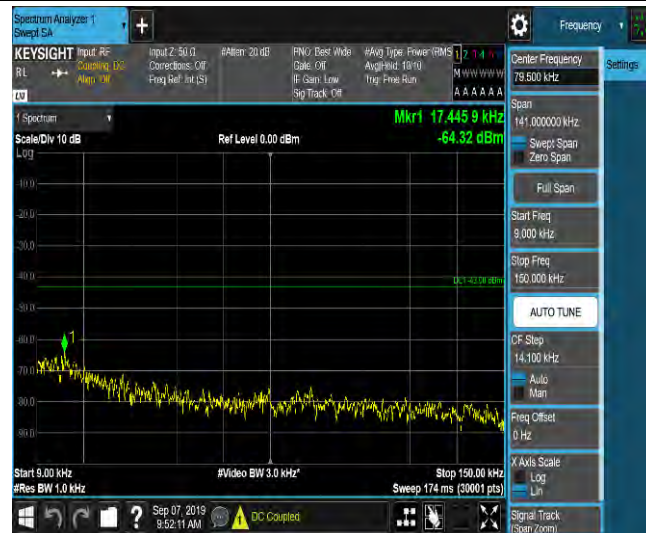
LTE Band 2_3MHz_16QAM_19185_1RB#0_Range2:0.15~30MHz_-60.05_PASS
