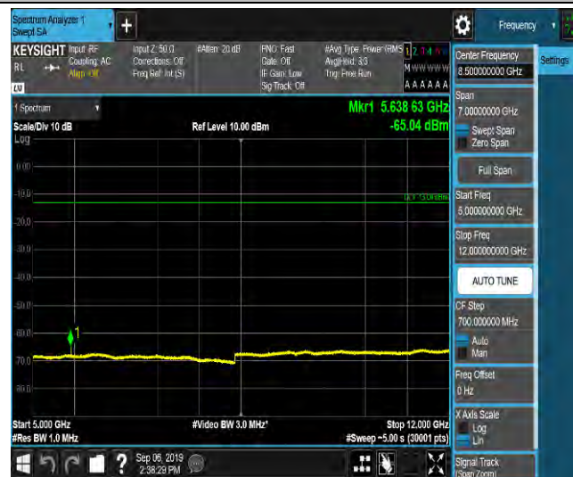
LTE Band 2_1.4MHz_QPSK_18900_1RB#0_Range6:12000~18000MHz_-55.35_PASS
