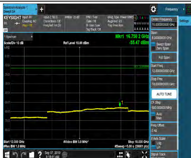
LTE Band 2_10MHz_QPSK_18900_1RB#0_Range1:0.009~0.15MHz_-63.76_PASS
