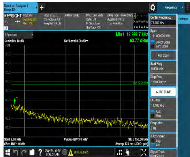
LTE Band 2_5MHz_16QAM_18900_1RB#0_Range2:0.15~30MHz_-59.93_PASS
