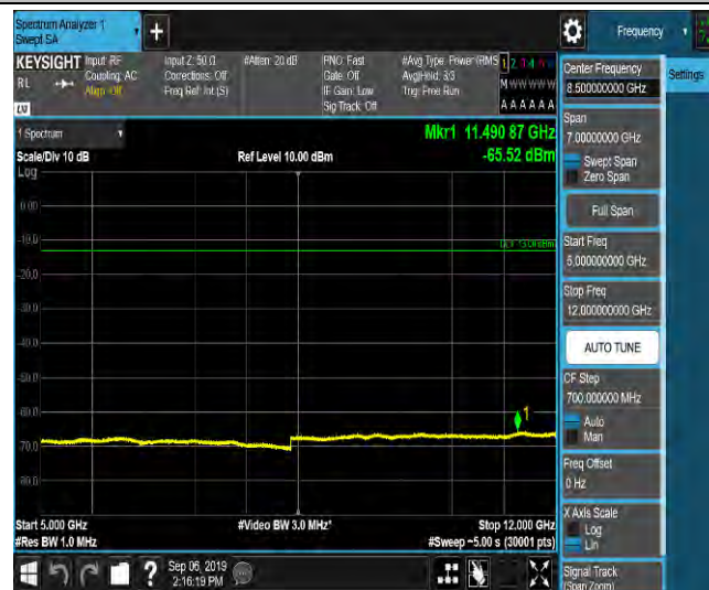
LTE Band 2_1.4MHz_QPSK_18607_1RB#0_Range6:12000~18000MHz_-55.35_PASS
