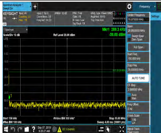
LTE Band 2_10MHz_QPSK_19150_1RB#0_Range3:30~1000MHz_-46.61_PASS
