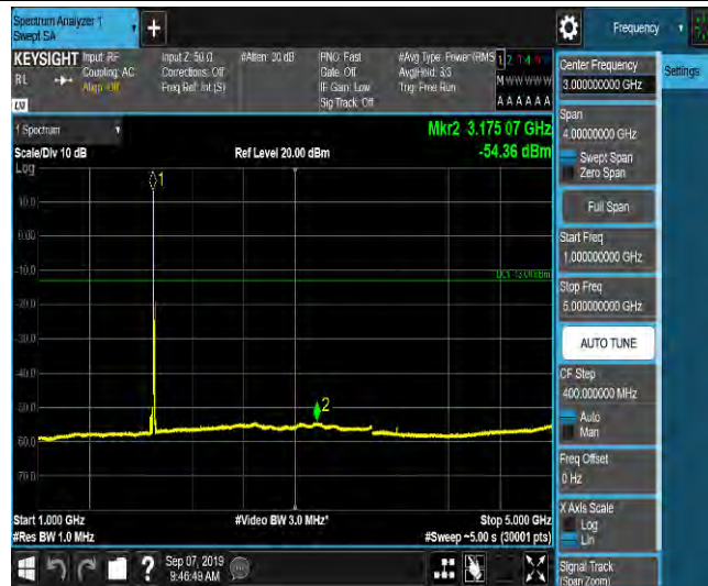
LTE Band 2_15MHz_16QAM_19125_1RB#0_Range5:5000~12000MHz_-65.52_PASS
