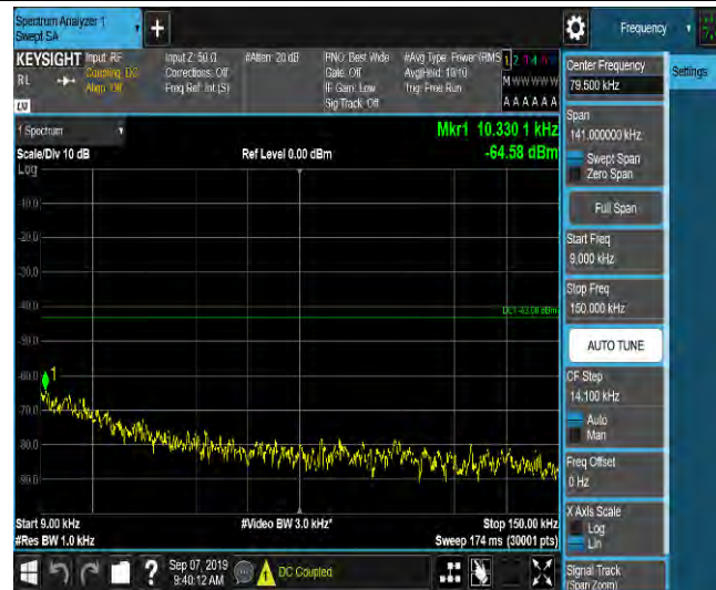
LTE Band 2_15MHz_16QAM_18675_1RB#0_Range2:0.15~30MHz_-60.41_PASS
