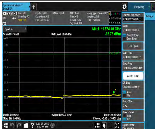
LTE Band 2_15MHz_16QAM_18900_1RB#0_Range6:12000~18000MHz_-55.52_PASS
