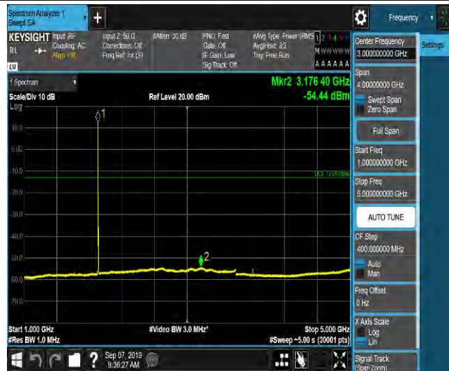
LTE Band 2_5MHz_16QAM_19175_1RB#0_Range5:5000~12000MHz_-64.94_PASS
