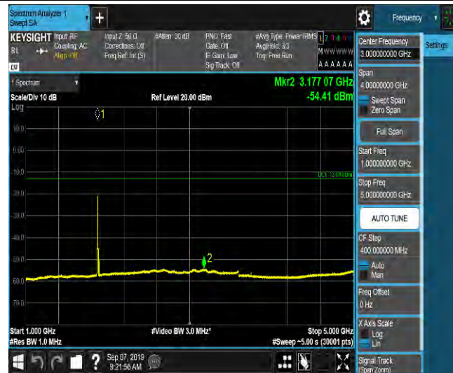
LTE Band 2_10MHz_QPSK_18900_1RB#0_Range5:5000~12000MHz_-65.47_PASS
