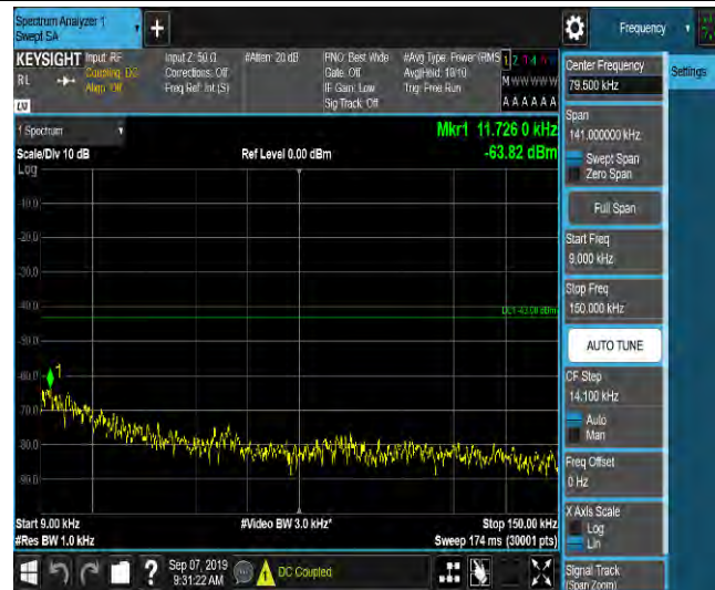
LTE Band 2_5MHz_QPSK_18900_1RB#0_Range2:0.15~30MHz_-59.72_PASS
