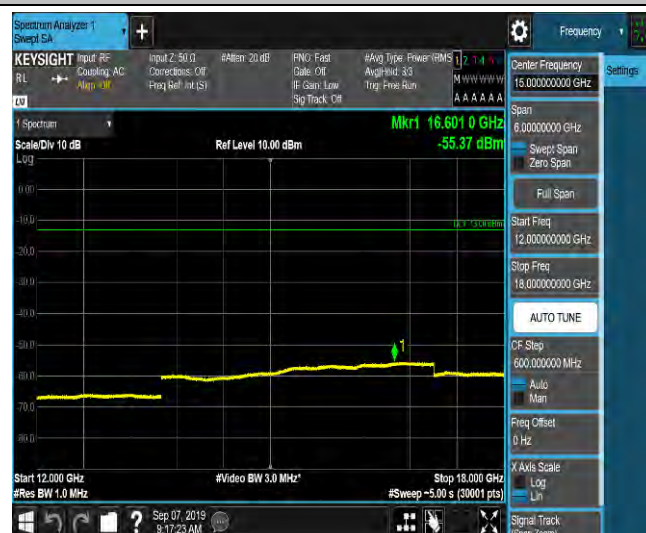
LTE Band 2_10MHz_16QAM_18650_1RB#0_Range1:0.009~0.15MHz_-62.83_PASS
