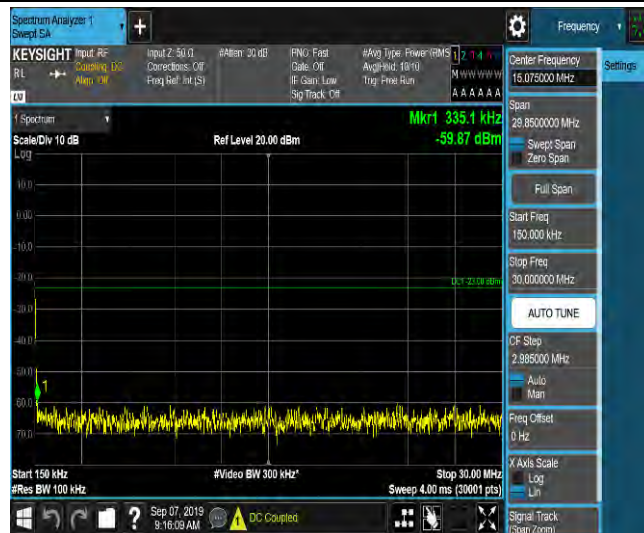
LTE Band 2_10MHz_QPSK_18650_1RB#0_Range3:30~1000MHz_-47.53_PASS
