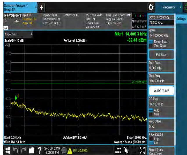
LTE Band 2_1.4MHz_QPSK_19193_1RB#0_Range2:0.15~30MHz_-57.76_PASS
