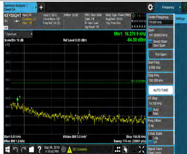
LTE Band 2_3MHz_QPSK_18615_1RB#0_Range2:0.15~30MHz_-57.86_PASS
