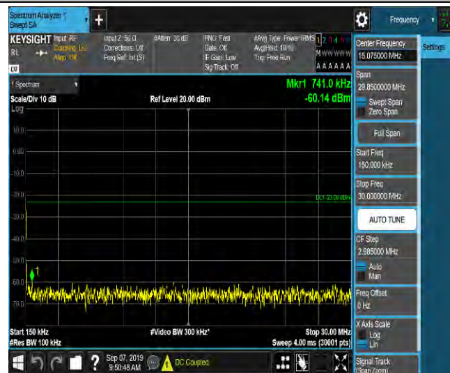
LTE Band 2_3MHz_QPSK_19185_1RB#0_Range3:30~1000MHz_-47.28_PASS
