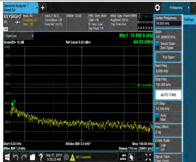
LTE Band 2_5MHz_QPSK_18625_1RB#0_Range2:0.15~30MHz_-58.77_PASS
