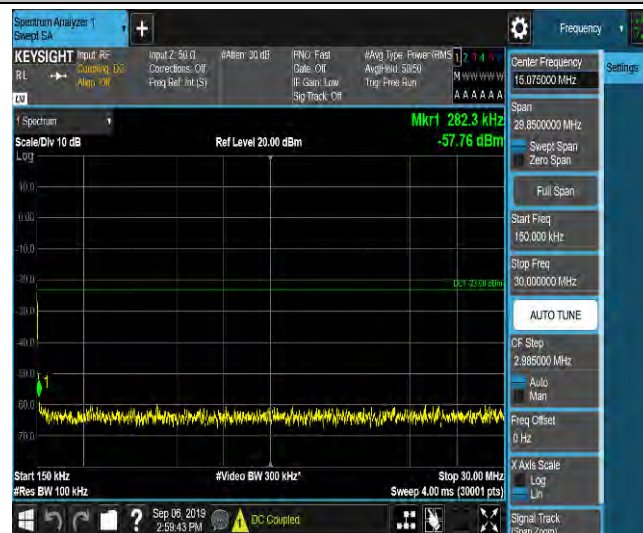
LTE Band 2_1.4MHz_QPSK_19193_1RB#0_Range3:30~1000MHz_-46.1_PASS
