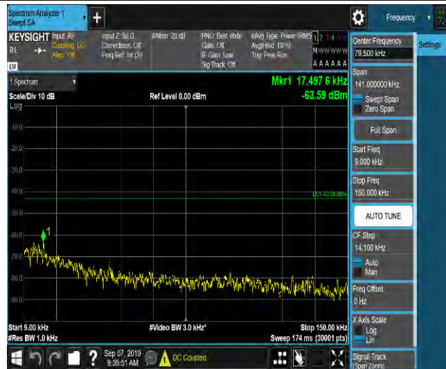
LTE Band 2_5MHz_16QAM_19175_1RB#0_Range2:0.15~30MHz_-58.65_PASS
