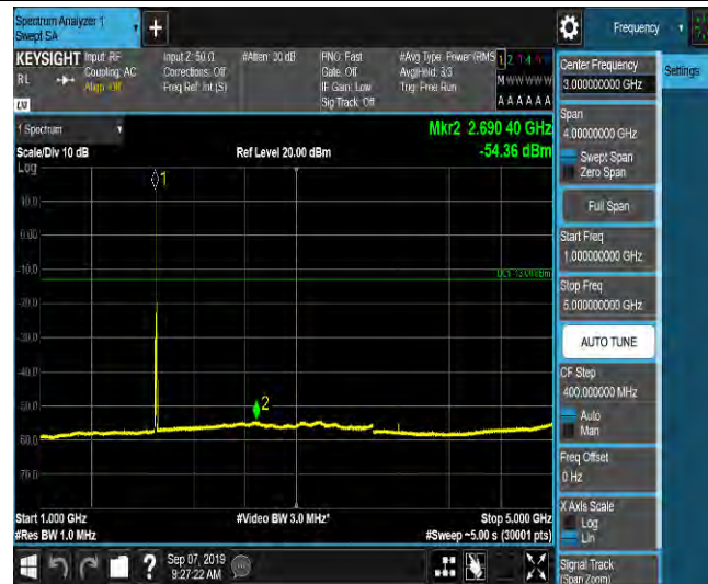
LTE Band 2_10MHz_16QAM_19150_1RB#0_Range5:5000~12000MHz_-65.29_PASS
