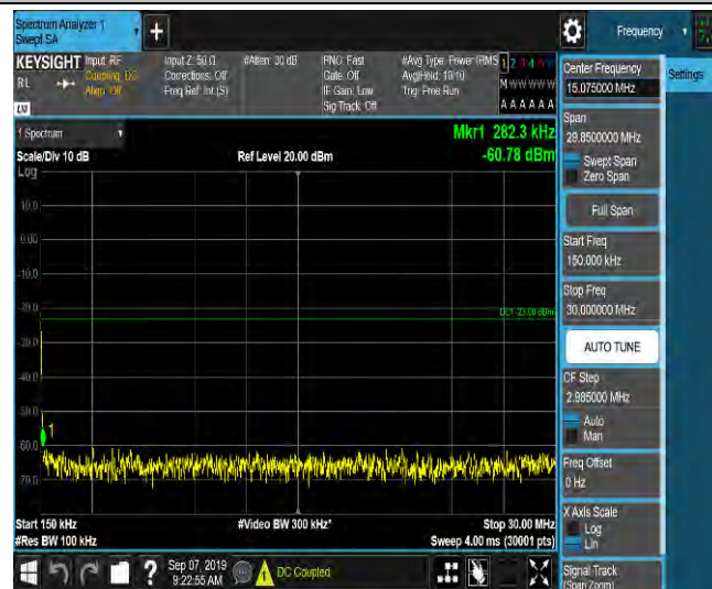
LTE Band 2_10MHz_16QAM_18900_1RB#0_Range3:30~1000MHz_-46.56_PASS
