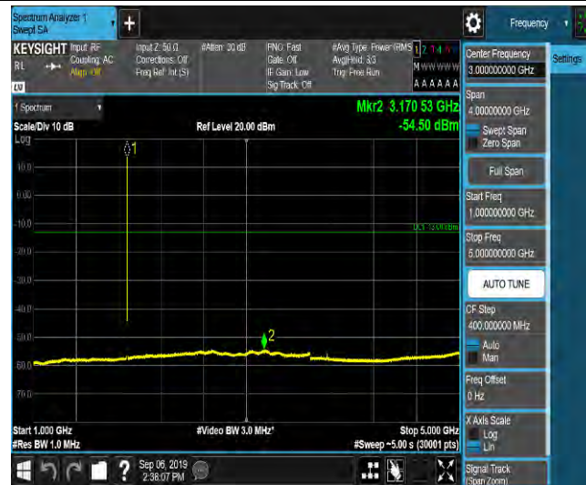
LTE Band 2_1.4MHz_QPSK_18900_1RB#0_Range5:5000~12000MHz_-65.05_PASS
