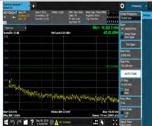
LTE Band 2_3MHz_16QAM_18615_1RB#0_Range2:0.15~30MHz_-59.5_PASS
