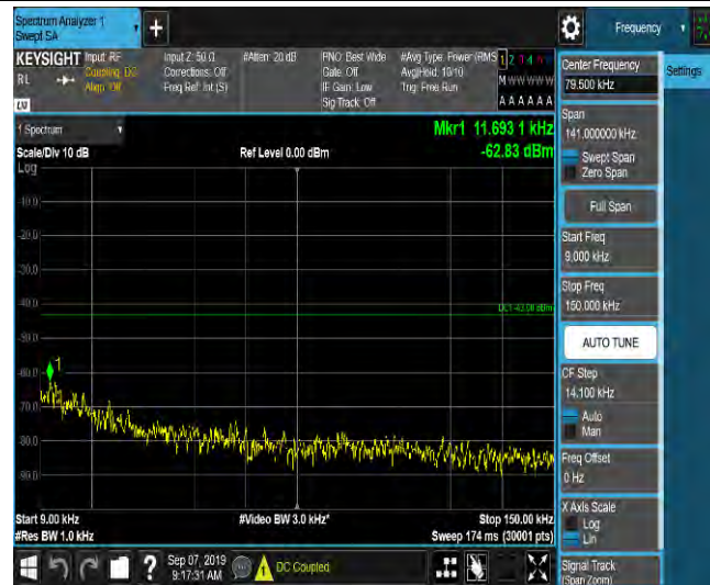
LTE Band 2_10MHz_16QAM_18650_1RB#0_Range2:0.15~30MHz_-60.42_PASS
