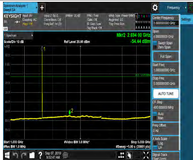
LTE Band 2_3MHz_16QAM_19185_1RB#0_Range5:5000~12000MHz_-63.72_PASS
