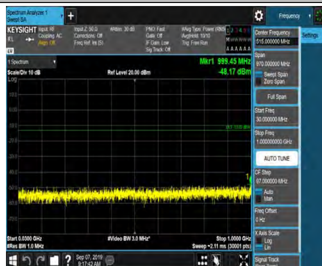
LTE Band 2_10MHz_16QAM_18650_1RB#0_Range4:1000~5000MHz_-54.28_PASS
