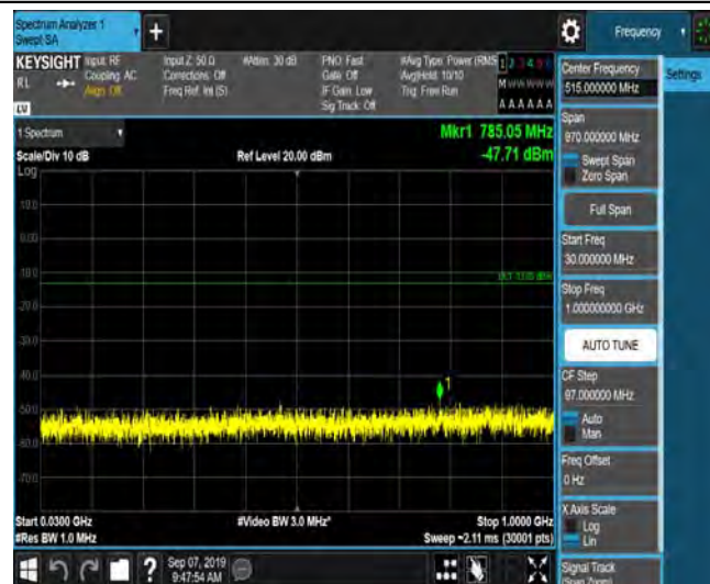
LTE Band 2_3MHz_QPSK_18900_1RB#0_Range4:1000~5000MHz_-54.29_PASS
