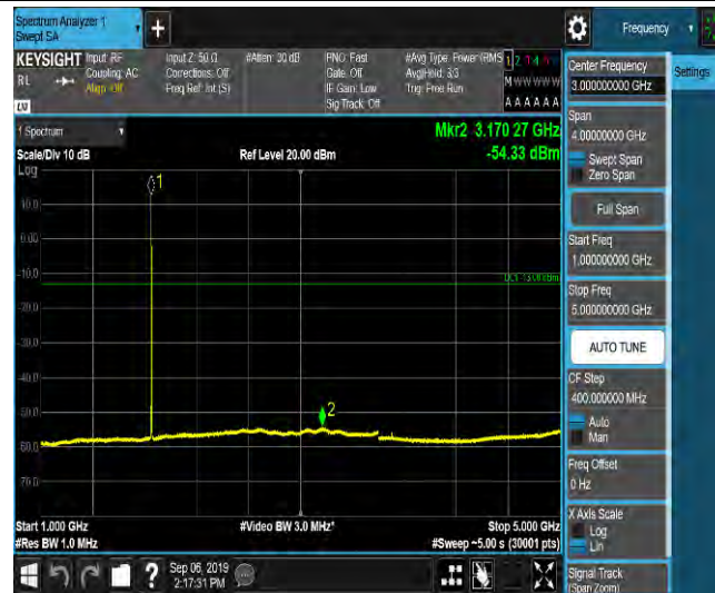
LTE Band 2_1.4MHz_16QAM_18607_1RB#0_Range5:5000~12000MHz_-65.56_PASS
