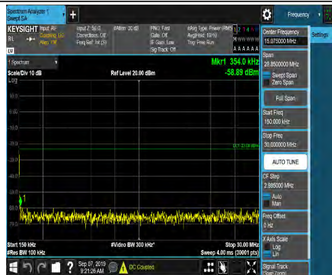
LTE Band 2_10MHz_QPSK_18900_1RB#0_Range3:30~1000MHz_-46.89_PASS
