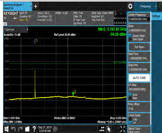
LTE Band 2_10MHz_16QAM_18900_1RB#0_Range5:5000~12000MHz_-65.69_PASS
