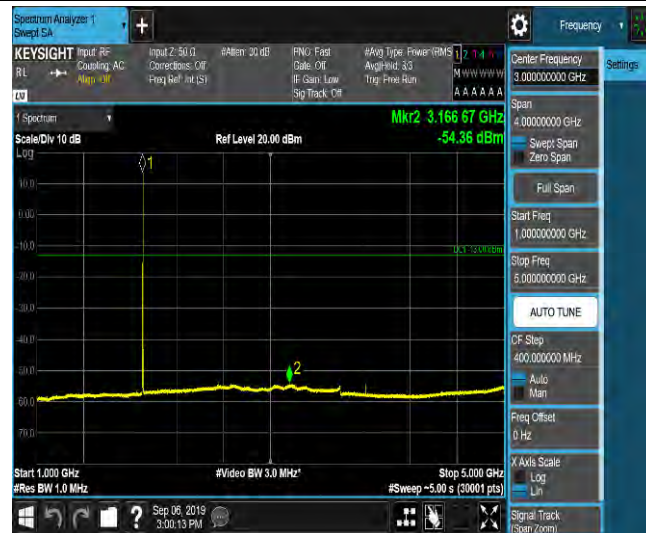
LTE Band 2_1.4MHz_QPSK_19193_1RB#0_Range5:5000~12000MHz_-63.23_PASS
