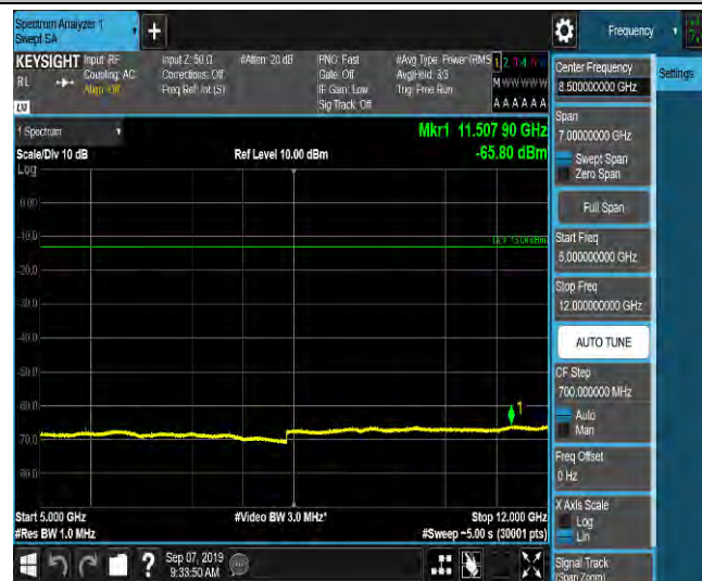
LTE Band 2_5MHz_16QAM_18900_1RB#0_Range6:12000~18000MHz_-55.48_PASS
