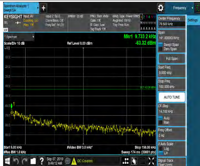
LTE Band 2_3MHz_16QAM_18900_1RB#0_Range2:0.15~30MHz_-57.64_PASS
