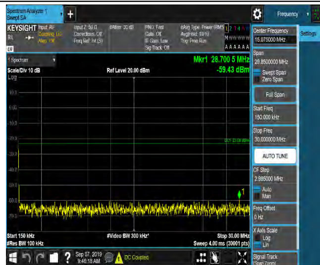
LTE Band 2_15MHz_16QAM_19125_1RB#0_Range3:30~1000MHz_-45.92_PASS
