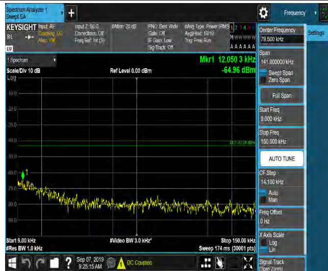
LTE Band 2_10MHz_QPSK_19150_1RB#0_Range2:0.15~30MHz_-59_PASS
