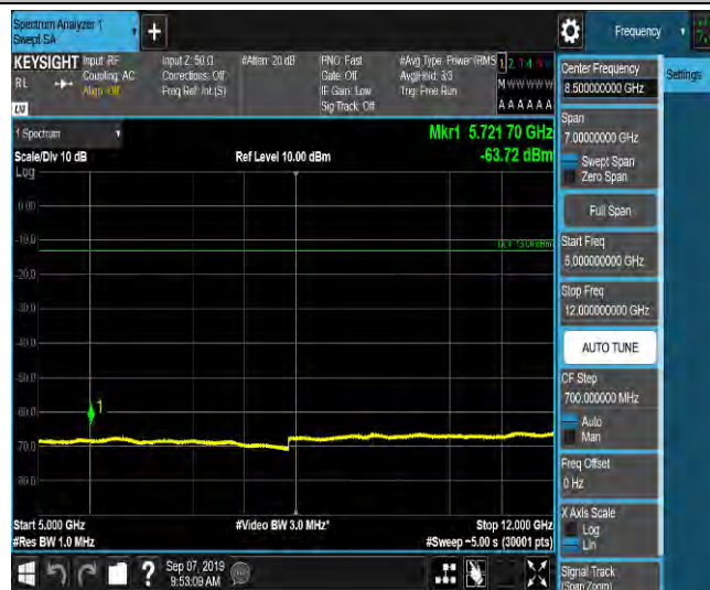
LTE Band 2_3MHz_16QAM_19185_1RB#0_Range6:12000~18000MHz_-55.47_PASS
