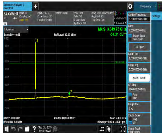
LTE Band 2_15MHz_QPSK_19125_1RB#0_Range5:5000~12000MHz_-64.48_PASS
