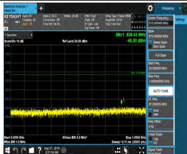
LTE Band 2_5MHz_QPSK_18900_1RB#0_Range4:1000~5000MHz_-54.34_PASS
