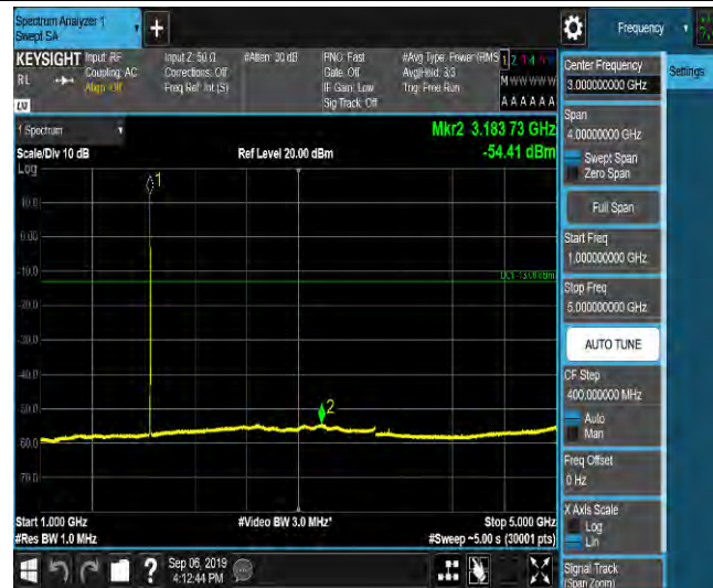
LTE Band 2_3MHz_16QAM_18615_1RB#0_Range5:5000~12000MHz_-65.7_PASS
