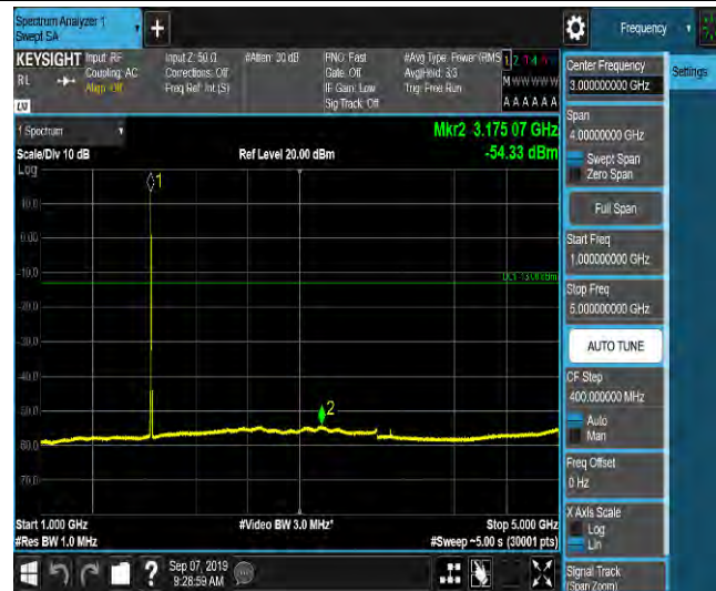
LTE Band 2_5MHz_QPSK_18625_1RB#0_Range5:5000~12000MHz_-65.85_PASS
