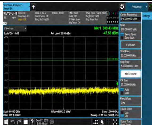
LTE Band 2_15MHz_QPSK_19125_1RB#0_Range4:1000~5000MHz_-54.31_PASS
