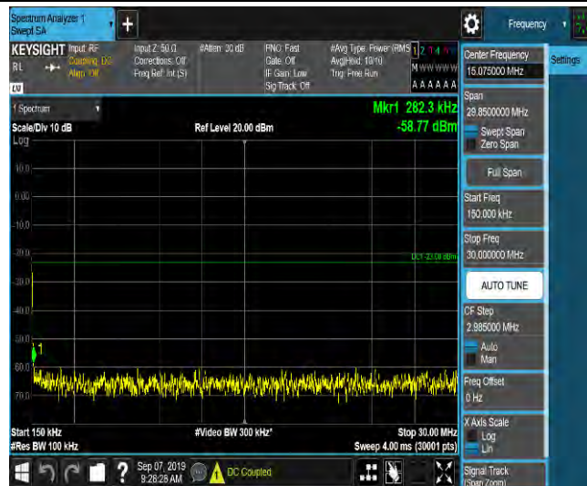
LTE Band 2_5MHz_QPSK_18625_1RB#0_Range3:30~1000MHz_-46.93_PASS
