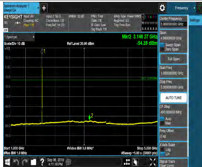
LTE Band 2_3MHz_QPSK_18615_1RB#0_Range5:5000~12000MHz_-65.64_PASS
