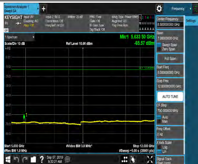
LTE Band 2 5MHz QPSK 18900 1RB#0 Range6:12000~18000MHz -55.43 PASS
