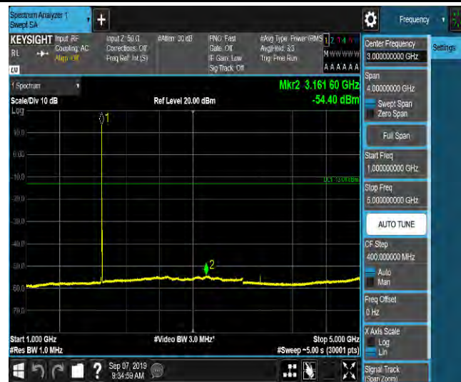
LTE Band 2_5MHz_QPSK_19175_1RB#0_Range5:5000~12000MHz_-63.86_PASS
