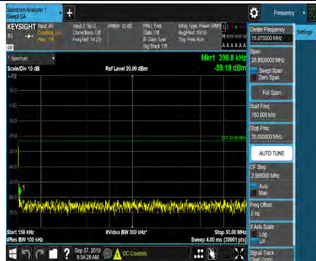
LTE Band 2_5MHz_QPSK_19175_1RB#0_Range3:30~1000MHz_-47.53_PASS
