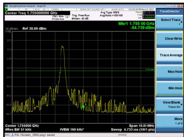
LTE Band 4 20MHz 16QAM 1RB CH-High
