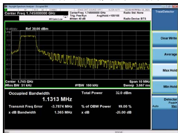
LTE Band 85 10MHz QPSK CH-Middle
