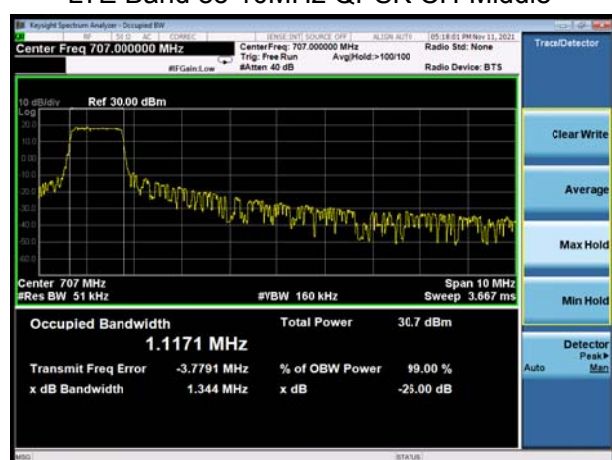
LTE Band 85 10MHz QPSK CH-Middle
