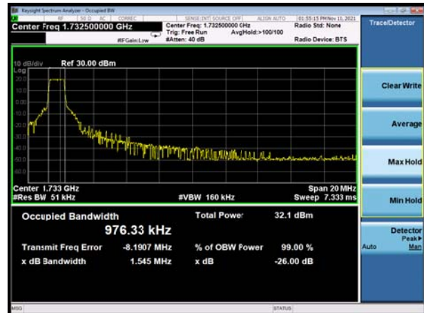
LTE Band 12 5MHz 16QAM CH-Middle
