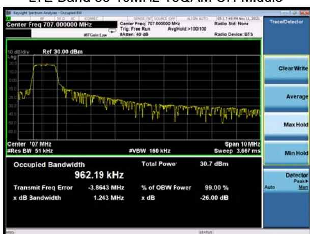
LTE Band 85 10MHz 16QAM CH-Middle
