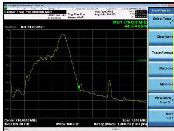
NB-IoT Band 85 QPSK 15kHz 12@0 CH-High
