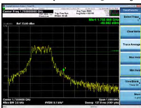
NB-IoT Band 4 QPSK 15kHz 12@0 CH-High
