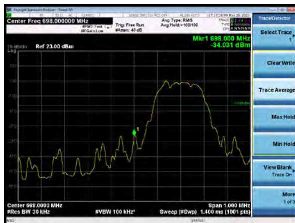
NB-IoT Band 85 QPSK 15kHz 12@0 CH-Low
