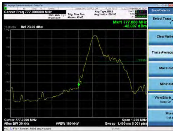
NB-IoT Band 13 QPSK 15kHz 12@0 CH-Low
