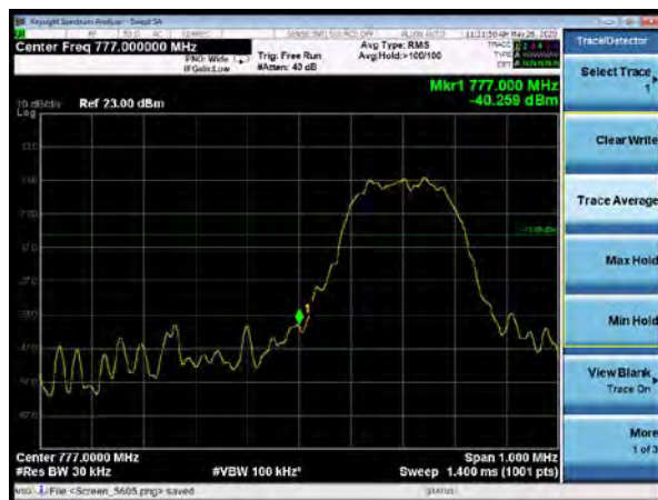
NB-IoT Band 13 QPSK 15kHz 12@0 CH-Low
