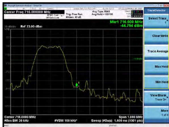
NB-IoT Band 85 QPSK 15kHz 12@0 CH-High
