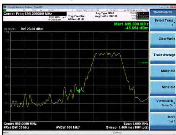
NB-IoT Band 12 QPSK 15kHz 12@0 CH-Low
