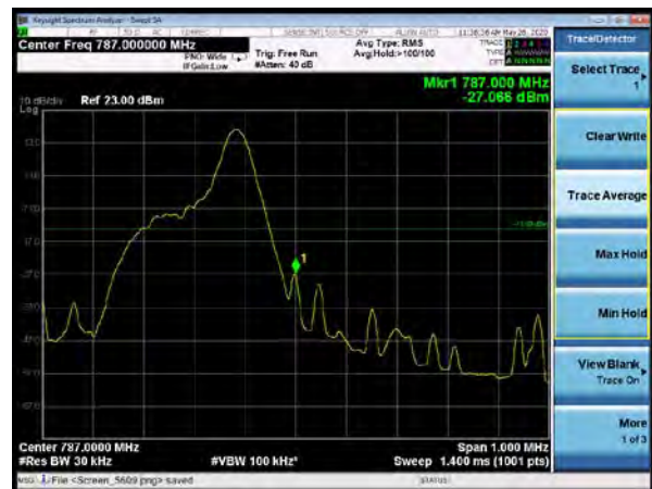
NB-IoT Band 13 QPSK 15kHz 12@0 CH-High
