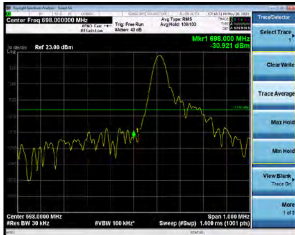
NB-IoT Band 85 QPSK 3.75kHz 1@0 CH-Low
