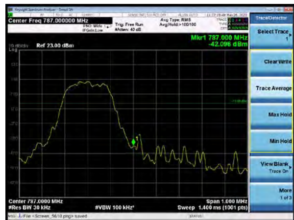
NB-IoT Band 13 QPSK 15kHz 12@0 CH-High
