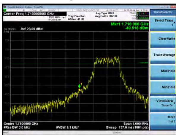
NB-IoT Band 66 QPSK 15kHz 12@0 CH-Low
