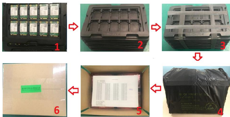
Figure 47: Tray Packaging Procedure
