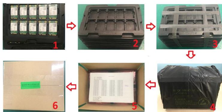
Figure 47: Tray Packaging Procedure
