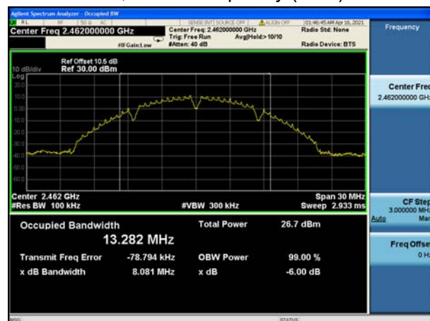
802.11b, Carrier frequency (MHz): 2462
