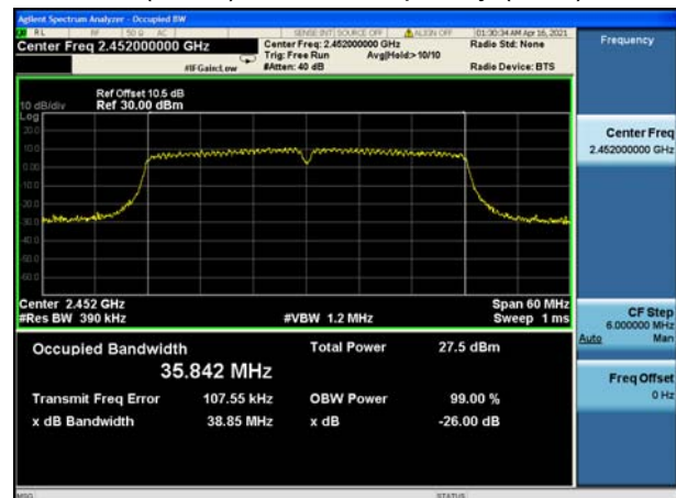
802.11n(HT40), Carrier frequency (MHz): 2452
