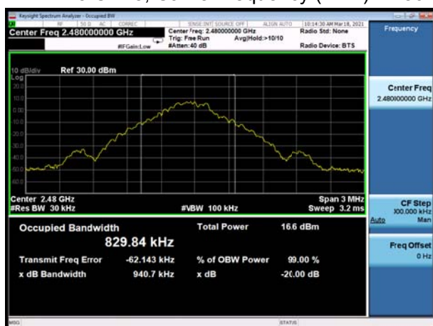
BT DH5 CH78, Carrier frequency (MHz): 2480
