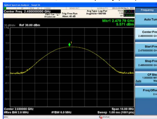
BT 2DH5 CH78, Carrier frequency (MHz): 2480
