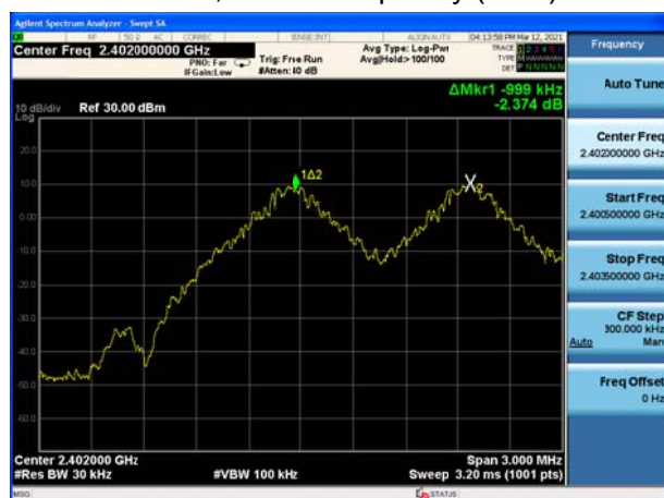
BT DH5 CH39, Carrier frequency (MHz): 2441
