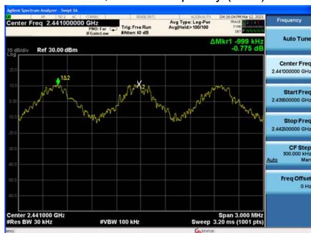
BT DH5 CH78, Carrier frequency (MHz): 2480
