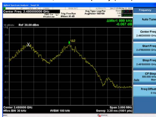
BT DH5 CH78, Carrier frequency (MHz): 2480
