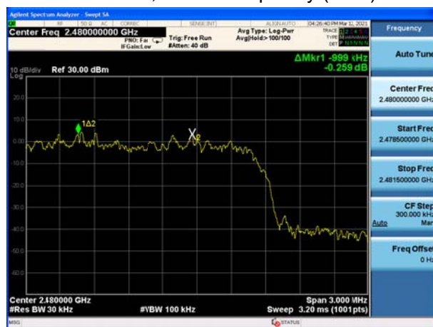
BT 2DH5 CH78, Carrier frequency (MHz): 2480
