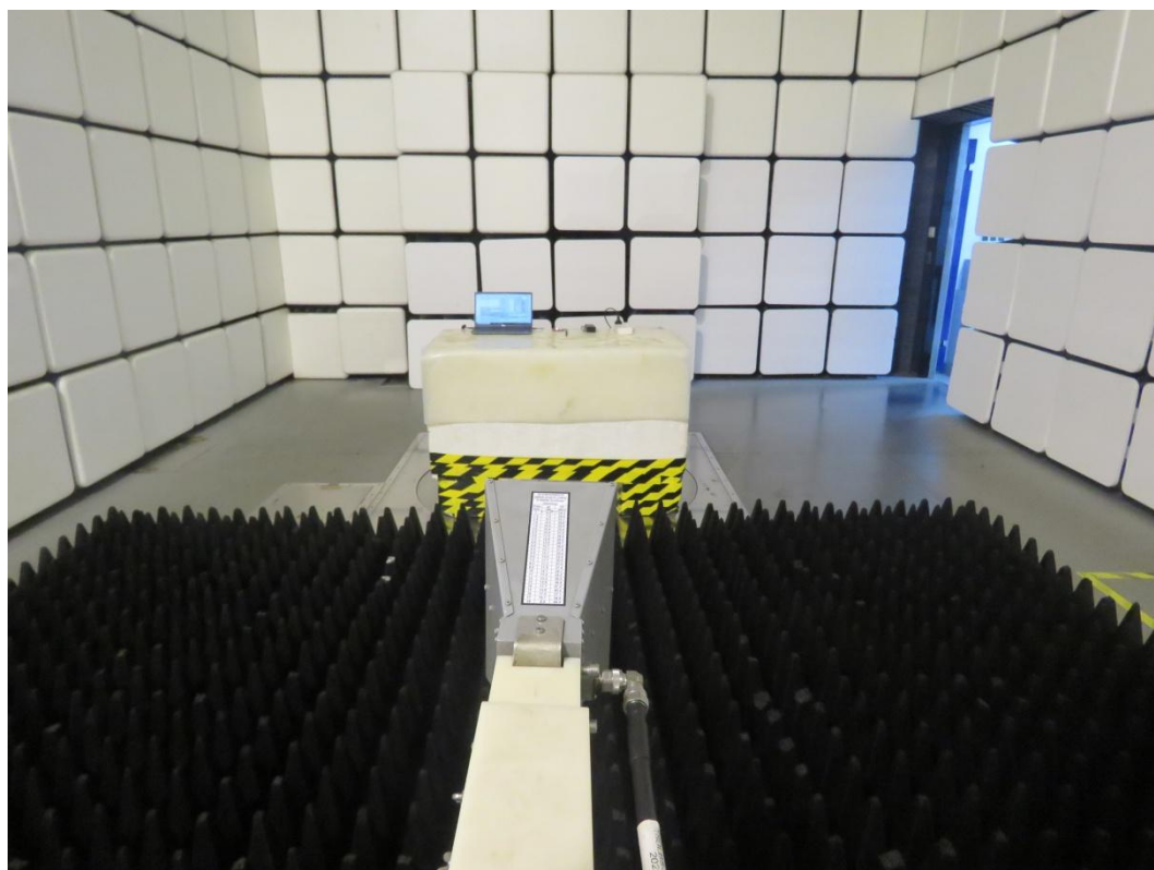
Picture 2: Receiver Spurious Emissions Test setup
