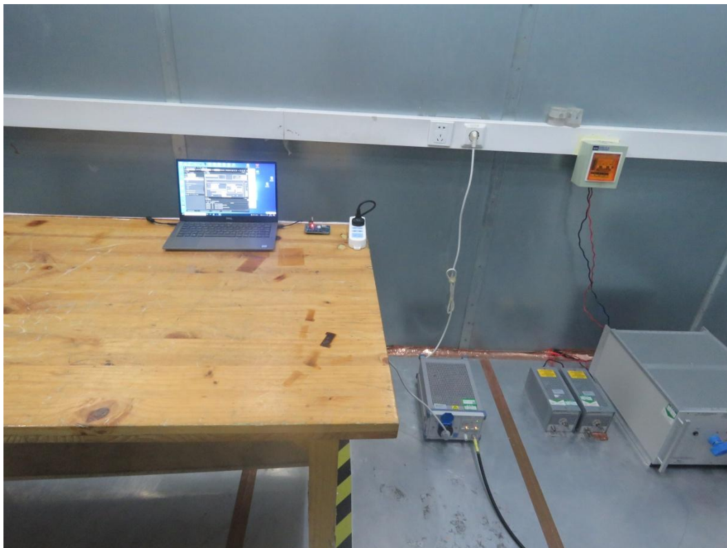
Picture 3: AC Power Line Conducted Emissions Test setup
