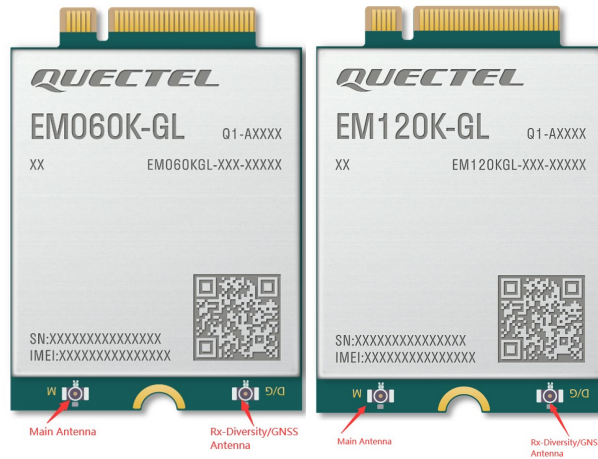
Figure 26: Antenna Connectors on the EM060K-GL and EM120K-GL
