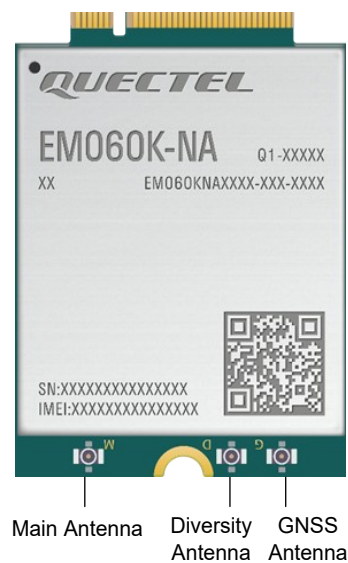
Figure 25: Antenna Connectors on EM060K-NA
