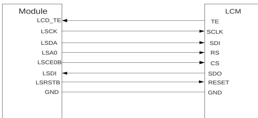
Figure 20: Reference Circuit Design for LCM Interface
