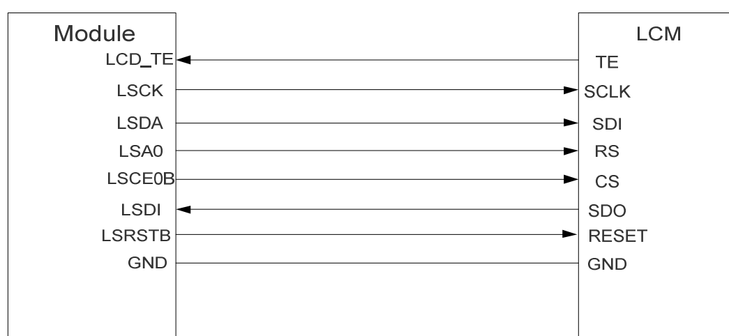
Figure 20: Reference Circuit Design for LCM Interface
