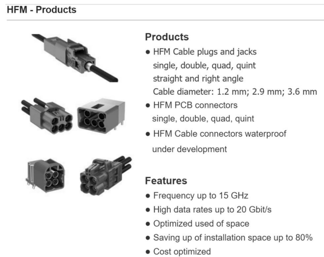
Figure 20: Description of the HFM Connector
