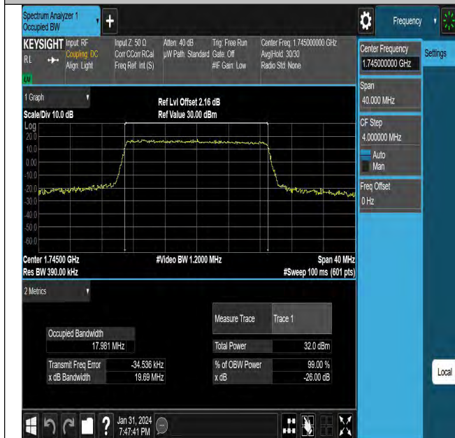
Band66-20MHz-QPSK-132322-100RB#0-PASS
